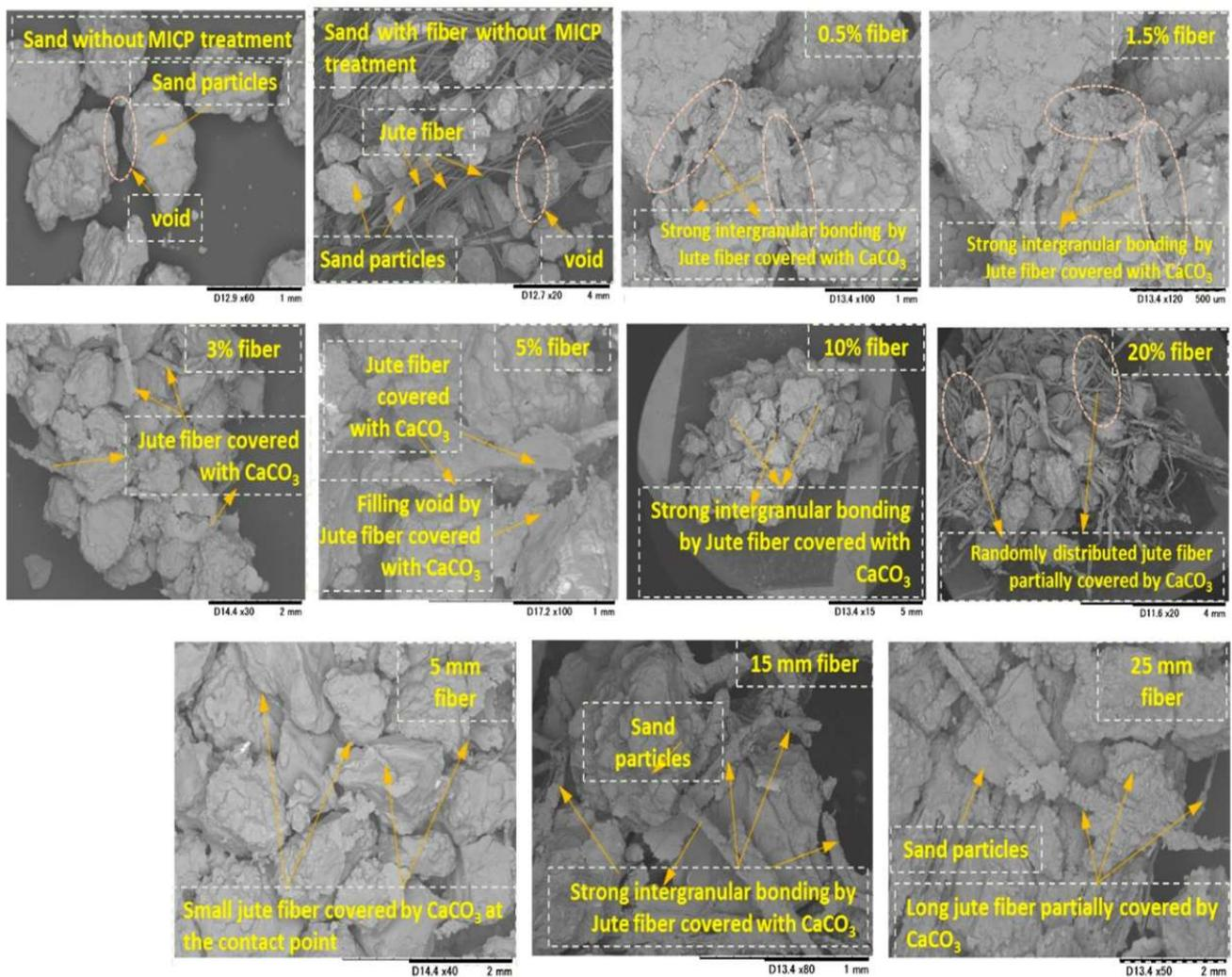
**Figure 5.** SEM images of MICP-treated bio-cemented samples with the addition of jute fibers (considering different lengths and contents) and distribution of  $\text{CaCO}_3$  within the sand matrix, reproduce with permission from [174].
