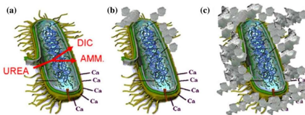
**Figure 2.** Schematic diagram (a) precursor intake through cell membrane for growth of bacteria (b) indicates the nucleation site and attachment of cationic ions and (c) suggests that urease-producing bacteria caused the calcium carbonate to precipitate. Reproduce with permission from [42].
