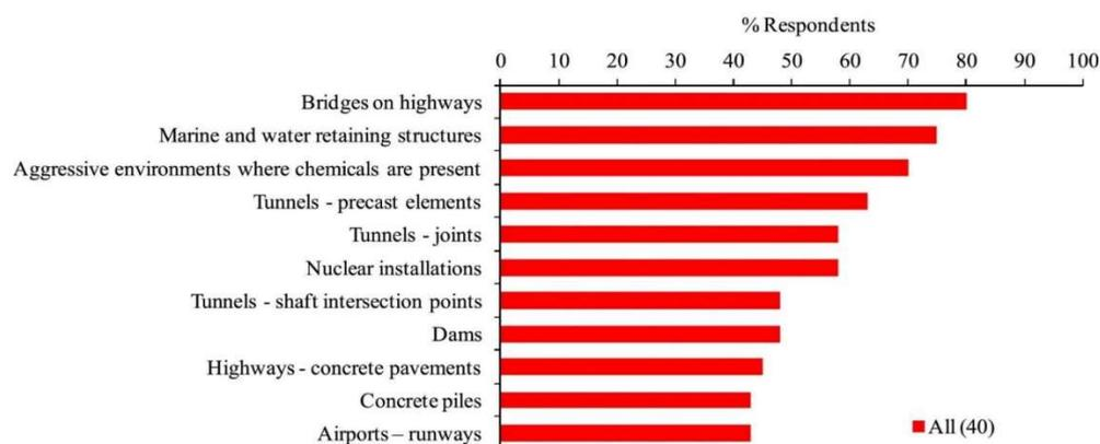
**Figure 7.** Proposed application areas of self healing bioconcrete [201].
