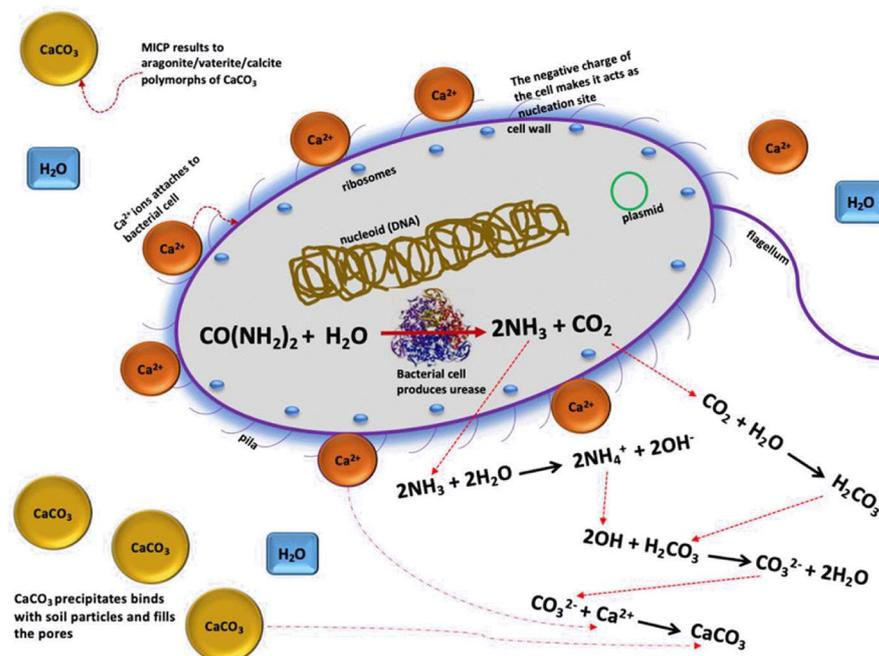
**Figure 1.** A diagram depicting the ureolytic bacterium *Sporosarcina pasteurii* in  $\text{CaCO}_3$  synthesis via the ureaolysis-driven microbially induced carbonate precipitation route for soil improvement. Reproduce with permission from publisher [37].
