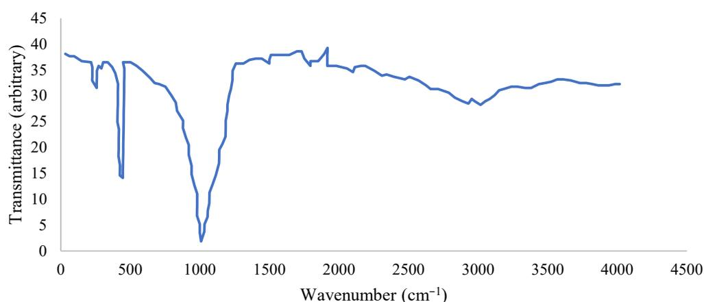
**Figure 6.** Portrays the FTIR spectral analysis of microbially induced  $\text{CaCO}_3$  modified and adaptive from [127].
