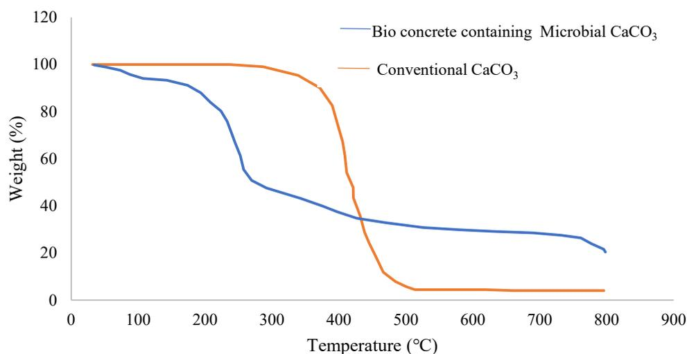
Figure 3. Demonstrates the TGA Analysis of bio-concrete [97].
