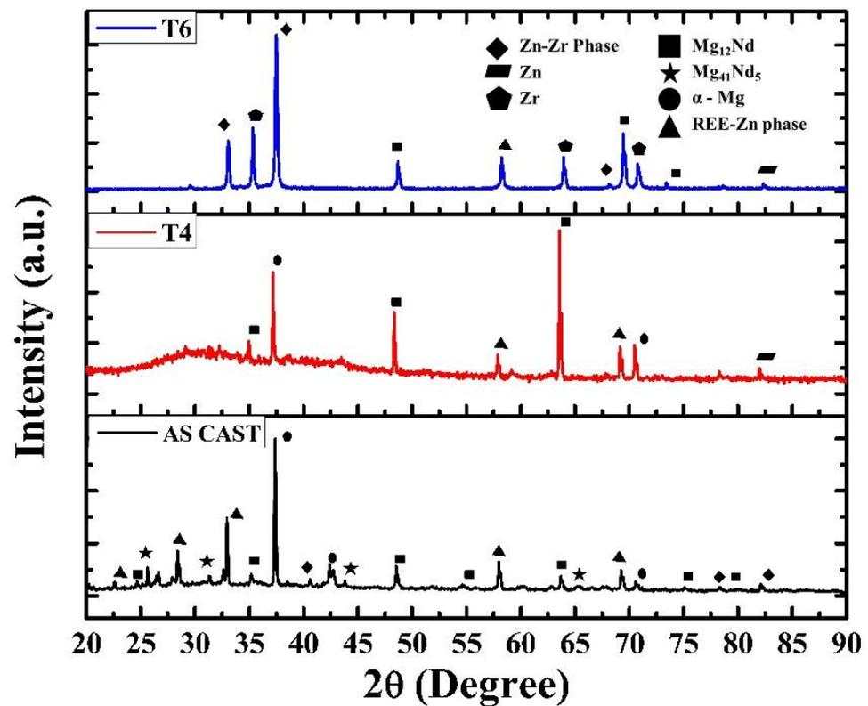
Figure 2. XRD patterns of EV31A in as-cast (black); T4 (red); T6 (blue) conditions.
