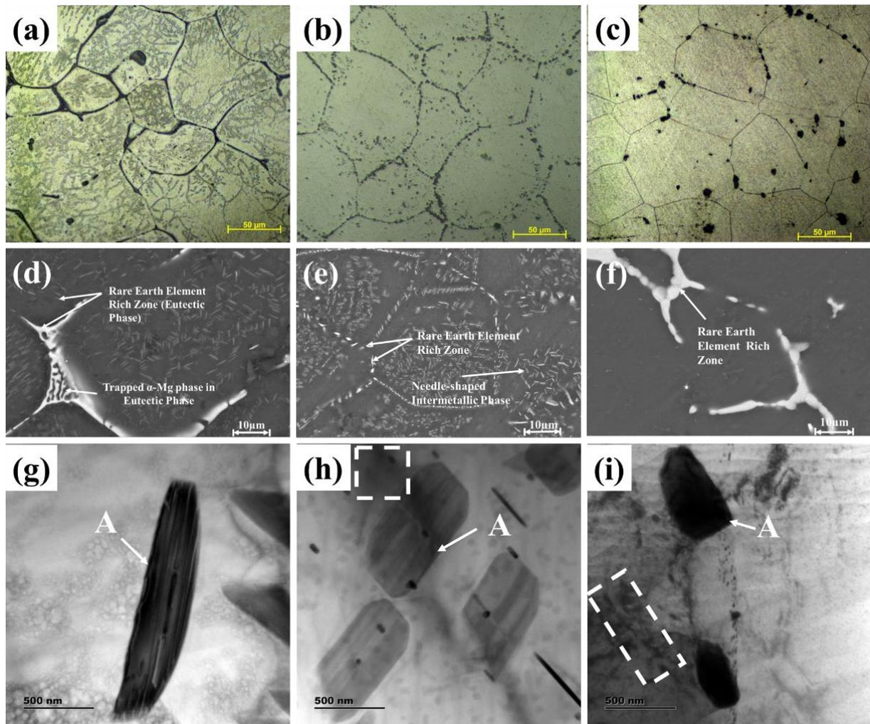
**Figure 3.** (a–c) Optical micrographs; (d–f) FE-SEM micrographs of EV31A; (g–i) Precipitates in studied alloy—TEM analysis. (a,d,g) As-cast; (b,e,h) after T4 heat-treatment; (c,f,i) after T6 heat-treatment. “A” point in Figure 3 (g–i) represents the precipitates, and the white rectangle in Figure 3 (h) and (i) represents dislocations.
