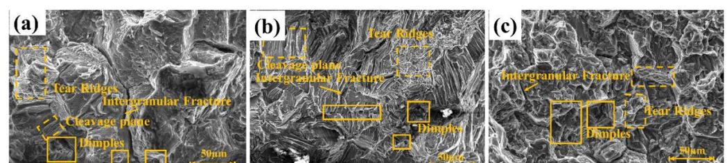
**Figure 5.** Fractography after tensile test of EV31A Mg alloy in SE mode of (a) As-cast; (b) T4, and (c) T6 conditions. (Solid rectangular box represents “Dimples”).
