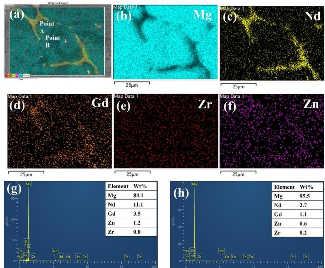
**Figure 4.** (a) SE micrograph of T6 heat-treated sample and EDS mapping of (b) Mg, (c) Nd, (d) Gd, (e) Zr, (f) Zn. EDS point analysis of (g) Point A and (h) Point B.
