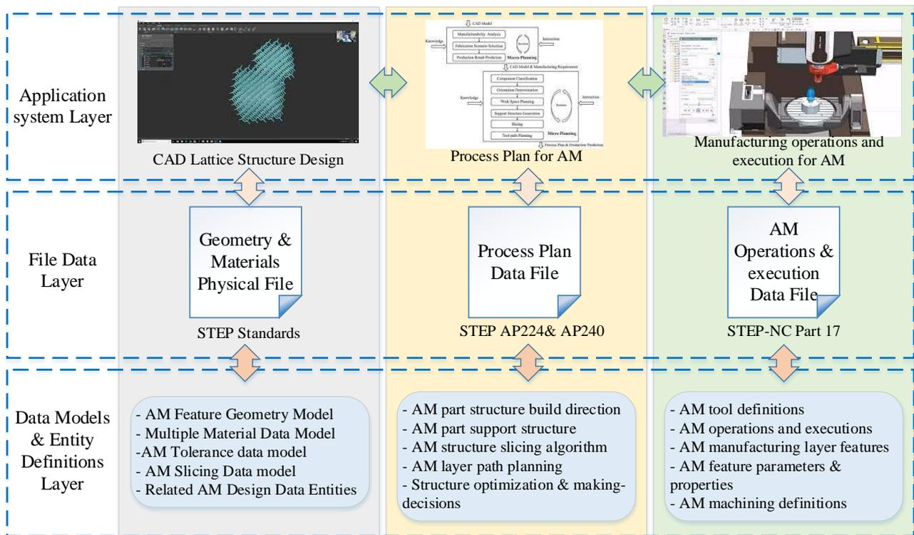
**Figure 1.** AM design and manufacturing information architecture based on various data layers.
