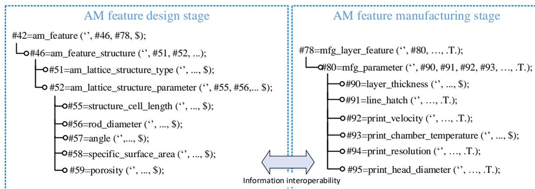
Figure 6. STEP physical file for AM feature design and manufacturing.
