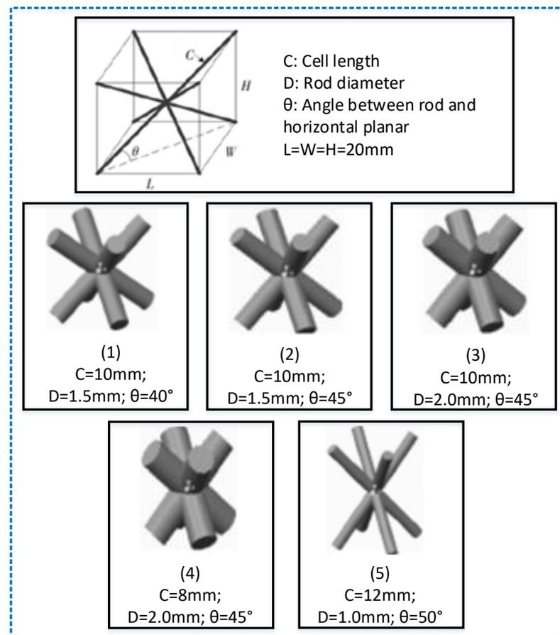
**Figure 2.** Comparison of different parameters for lattice structure.
