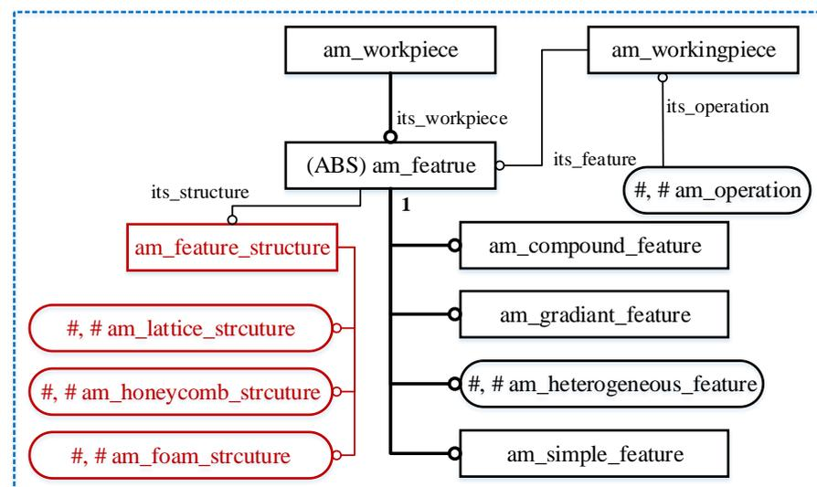
Figure 4. Extended STEP-compliant AM feature data model [15].
