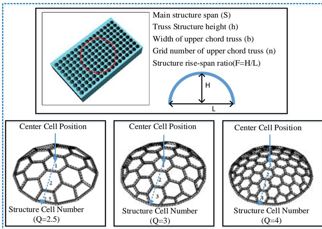
**Figure 3.** Honeycomb structure and related parameters.
