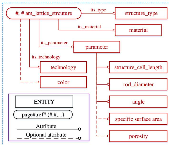
Figure 5. Data model for lattice structure based on EXPRESS-G.
