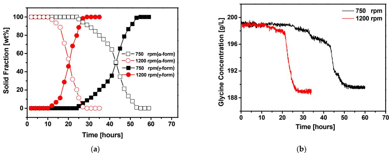
**Figure 4.** Influence of agitation speed on the polymorphic phase transformation of glycine  $\alpha$ -form to  $\gamma$ -form. (a) Solid fraction of  $\gamma$ -form and  $\alpha$ -form glycine; (b) glycine solution concentration during crystallization. The crystallization temperature, NaCl concentration, and seed concentration were fixed at 20 °C, 80 g/L, and 60 g/L, respectively.
