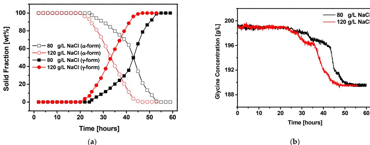
**Figure 6.** Influence of NaCl concentration on glycine polymorphic phase transformation of glycine  $\alpha$ -form to  $\gamma$ -form. (a) Solid fraction of  $\gamma$ -form and  $\alpha$ -form glycine; (b) glycine solution concentration during crystallization. The agitation speed, temperature, and seed concentration were fixed at 750 rpm, 20 °C, and 60 g/L, respectively.
