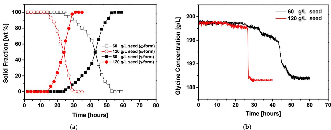
**Figure 7.** Influence of seed concentrations of  $\alpha$ -form on glycine polymorphic phase transformation of  $\alpha$ -form to  $\gamma$ -form. (a) Solid fraction of  $\gamma$ -form and  $\alpha$ -form glycine; (b) glycine solution concentration during crystallization. The agitation speed, temperature, and NaCl concentration were fixed at 750 rpm, 20 °C, and 80 g/L, respectively.
