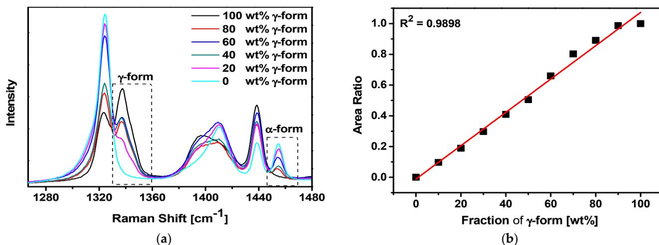
**Figure 3.** Analysis of the polymorphic fraction of glycine using FT-Raman spectroscopy: (a) comparison of characteristic relative peak intensities for the polymorphic mixture of  $\alpha$ -form and  $\gamma$ -form at various  $\gamma$ -form weight fractions; (b) standard calibration of  $\gamma$ -form characteristic peak area ratio and  $\gamma$ -form weight fraction in the polymorphic mixture of  $\alpha$ -form and  $\gamma$ -form.
