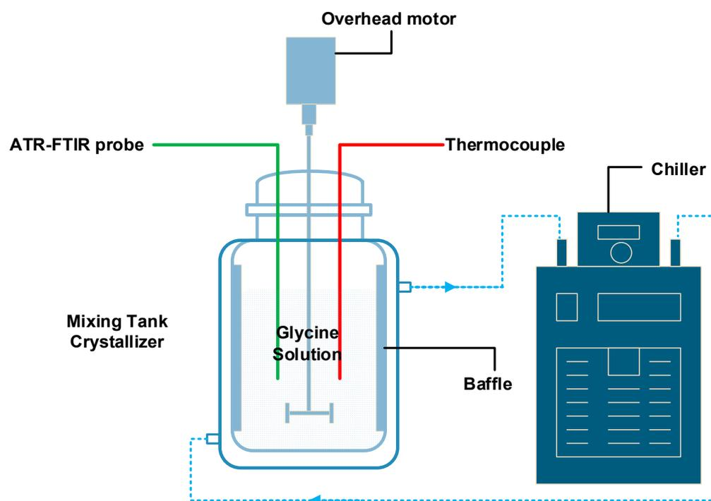
**Figure 1.** Schematic of the experimental setup in the mixing tank crystallizer consisting of in situ ATR-FTIR and a thermocouple probe.
