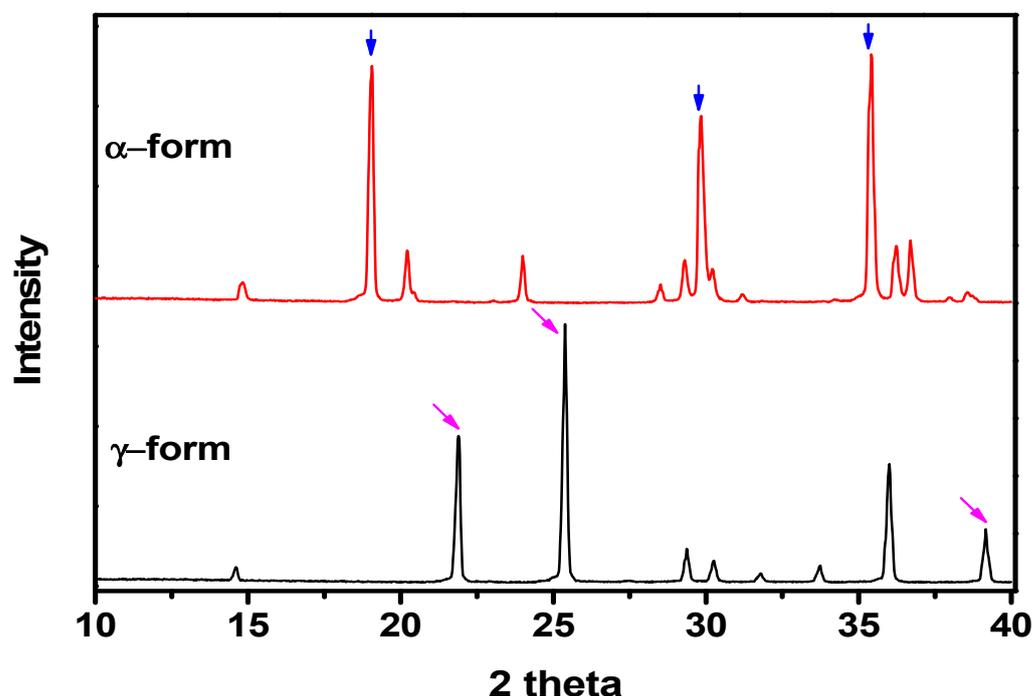
**Figure 2.** PXRD patterns of the  $\alpha$ -form and  $\gamma$ -form glycine crystals. The blue arrows indicate the characteristic peaks of  $\alpha$ -form ( $\sim 19.05^\circ$ ,  $\sim 29.9^\circ$ , and  $\sim 35.4^\circ$ ), and the pink arrows indicate the characteristic peaks of  $\gamma$ -form ( $\sim 21.8^\circ$ ,  $\sim 25.3^\circ$ , and  $\sim 39.1^\circ$ ).
