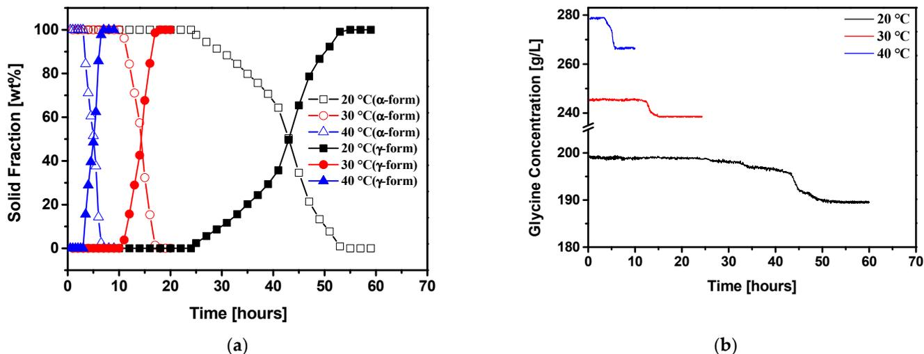
**Figure 5.** Influence of crystallization temperature on glycine polymorphic phase transformation of glycine  $\alpha$ -form to  $\gamma$ -form. (a) Solid fraction of  $\gamma$ -form and  $\alpha$ -form glycine; (b) glycine solution concentration during crystallization. The agitation speed, NaCl concentration, and seed concentration were fixed at 750 rpm, 80 g/L, and 60 g/L, respectively.
