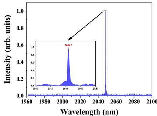
Figure 6. Spectrum of the Tm:YAG-Ho:GdVO<sub>4</sub> laser.
