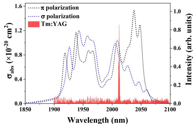
Figure 4. Output spectrum of the Tm:YAG laser and the absorption of the Ho:GdVO<sub>4</sub> crystal.
