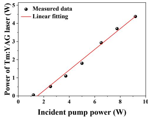
Figure 3. The output optical power of Tm:YAG laser varies with the incident pump.
