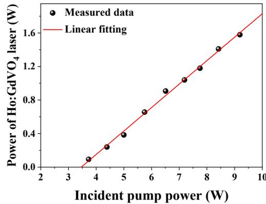
Figure 5. Power characteristics of the Tm:YAG-Ho:GdVO<sub>4</sub> laser.
