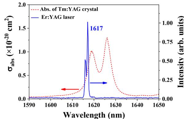
Figure 1. Absorption of the Tm:YAG crystal, including spectral curve of the Er:YAG laser.
