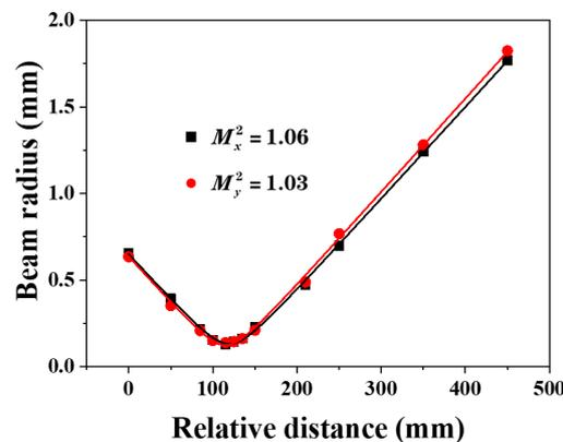
Figure 7.  $M^2$  measurement of the Tm:YAG-Ho:GdVO<sub>4</sub> laser.
