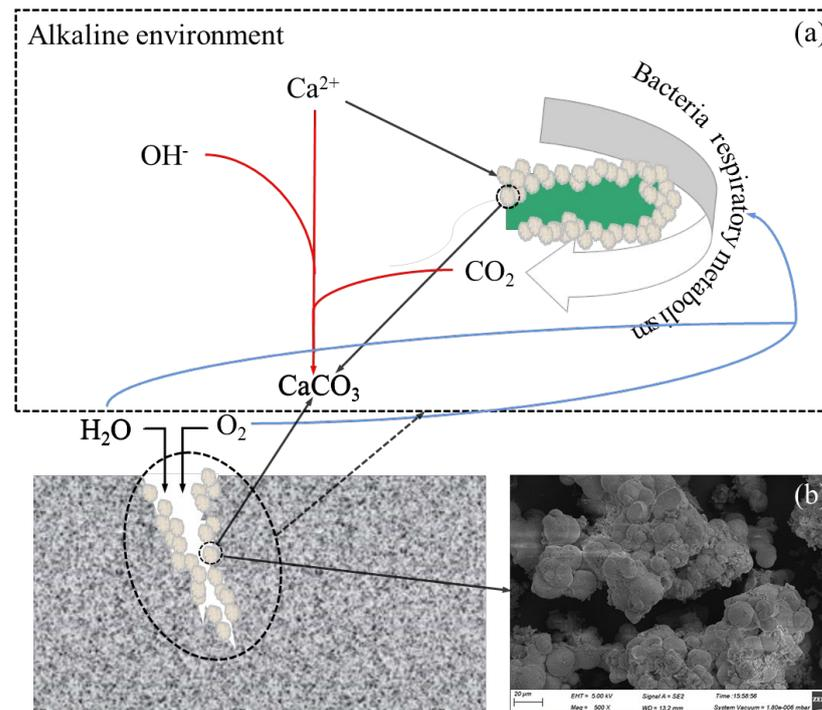
**Figure 1.** The principles and process of MICP technology for crack healing: (a) Microbially induced  $\text{CaCO}_3$  precipitation in cement-based material cracks; (b) Morphology of calcite formed by microbial induction.
