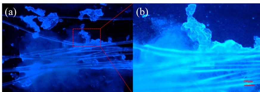
**Figure 4.** The optical microscope images of deposit on PP fiber [62]: (a) deposit induced by EPS; (b) biological organic film on PP fiber surface and deposits surface.
