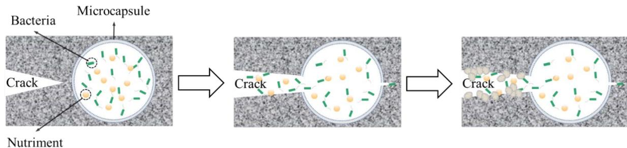
**Figure 5.** Schematic diagram of the self-healing process of microcapsules.
