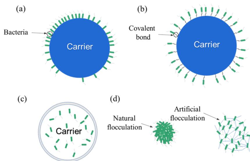
**Figure 2.** Microbial immobilization methods: (a) Adsorption; (b) Covalent binding; (c) Encapsulation; (d) Flocculation.
