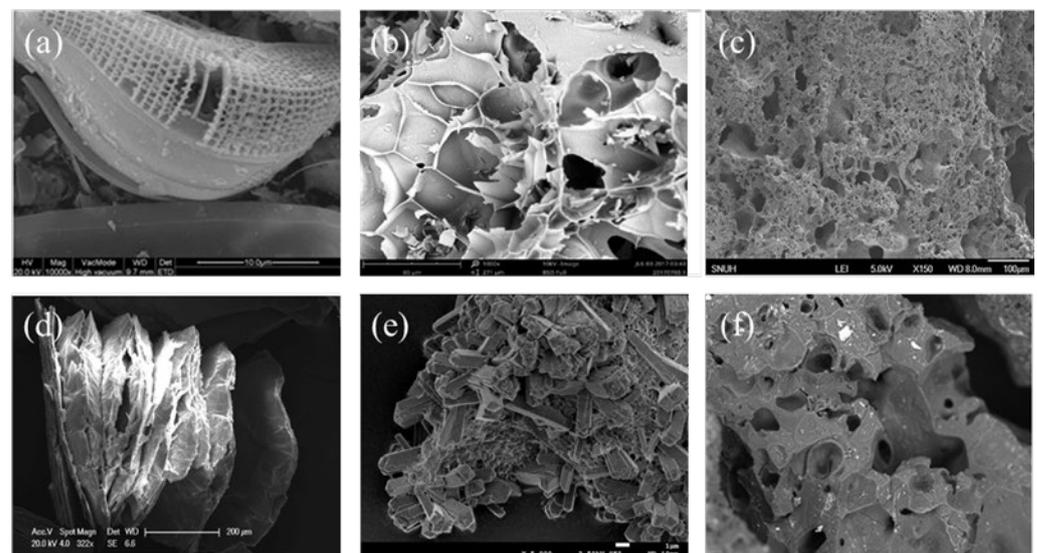
**Figure 3.** The microstructure of different materials: (a) diatomite [46]; (b) expanded perlite [42]; (c) expanded clay [43]; (d) expanded vermiculite [45]; (e) zeolite [47]; (f) granular activated carbon [48].
