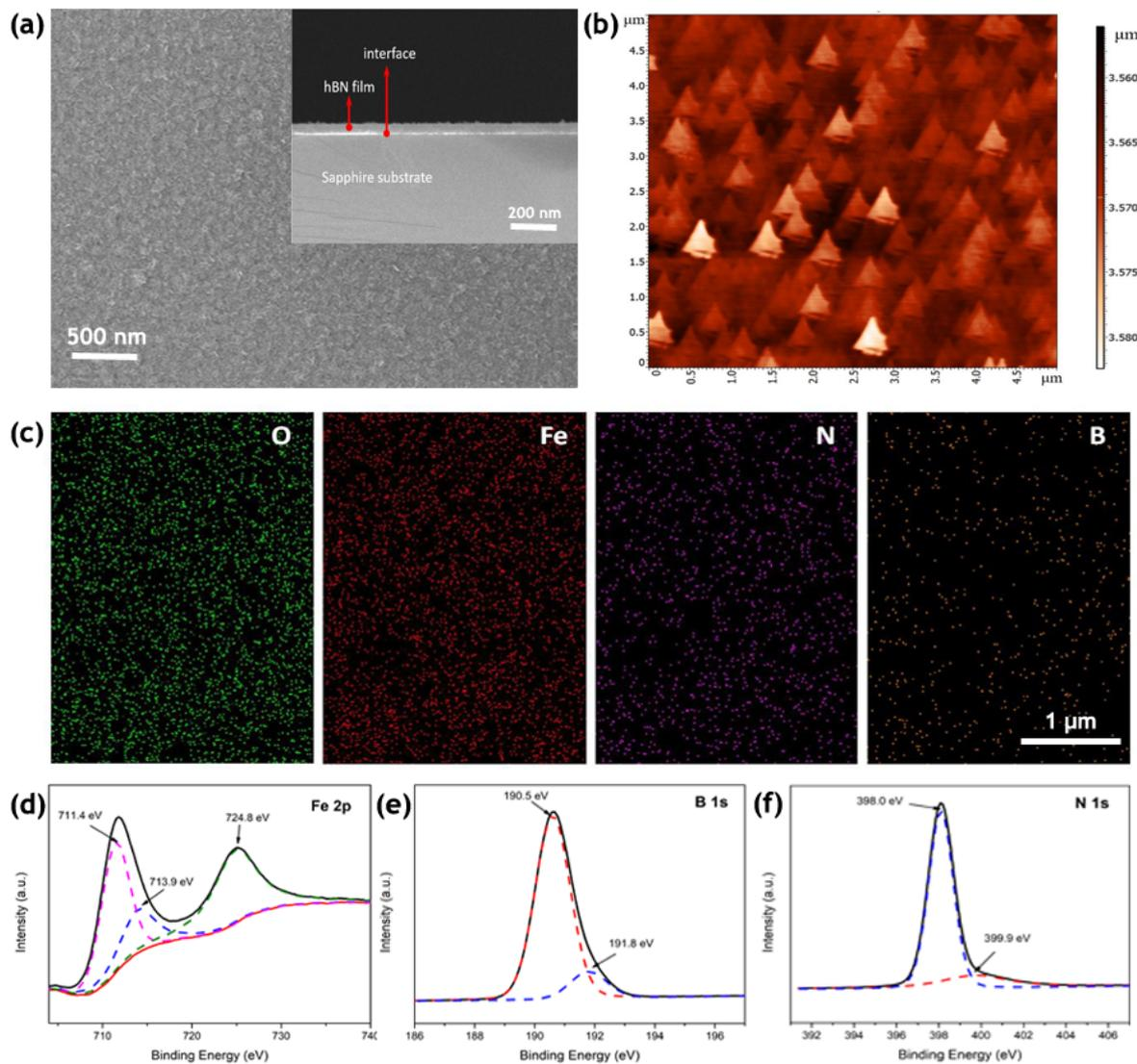
**Figure 1.** (a) The top view and the cross-sectional SEM images of Fe-doped hBN film. (b) The AFM image of Fe-doped hBN film ( $5\ \mu\text{m} \times 5\ \mu\text{m}$ ). (c) The distribution of element content from EDS. (d) The XPS spectra of Fe 2p, (e) B 1s, and (f) N 1s.
