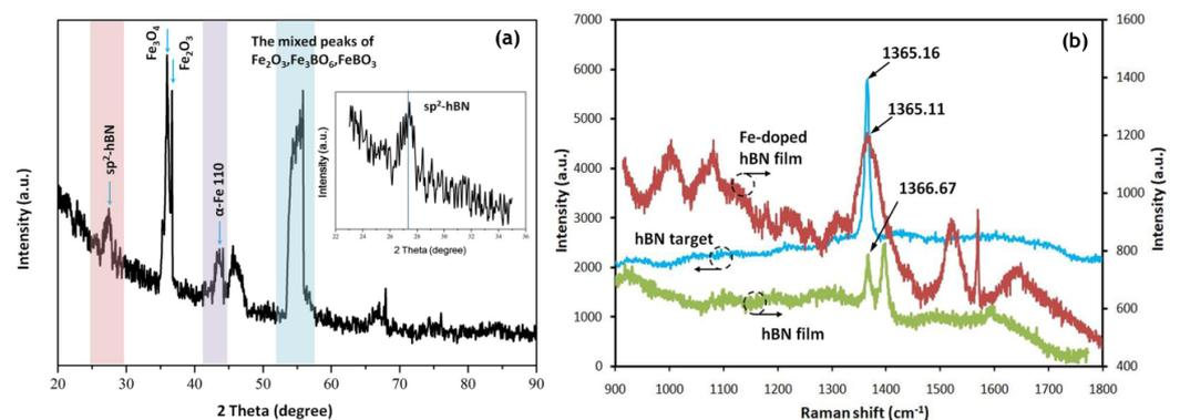
**Figure 3.** The (a) XRD patterns and (b) Raman spectra of Fe-doped hBN film.
