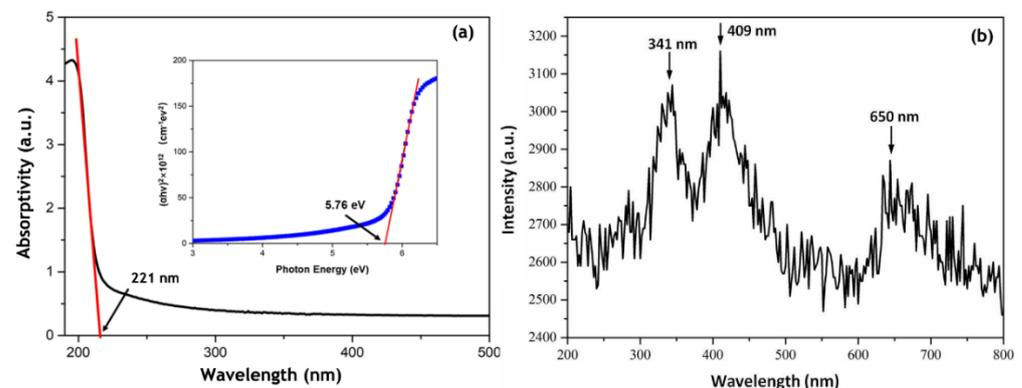
**Figure 4.** (a) The UV–Vis absorption spectrum (b) the CL spectrum of Fe–doped hBN film. The insert shows optical band gap (5.76 eV) analysis of Fe–doped hBN from the absorption spectrum.
