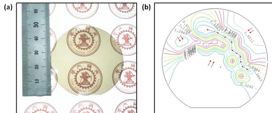
**Figure 2.** (a) Two inch wafer–scale film on sapphire with the thickness of 150 nm. (b) The square resistance mapping during the growth of thin film.
