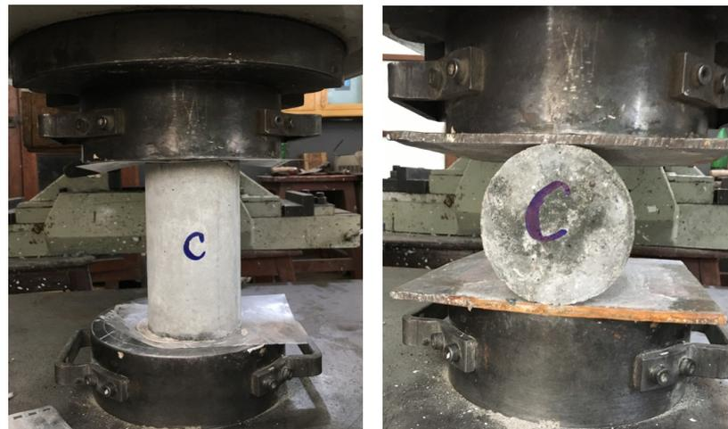
Figure 4. Test setup used to measure the compressive and tensile strength of concrete specimens.
