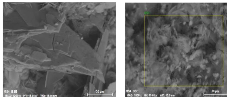
**Figure 10.** SEM image of cement paste with NC 6%.
