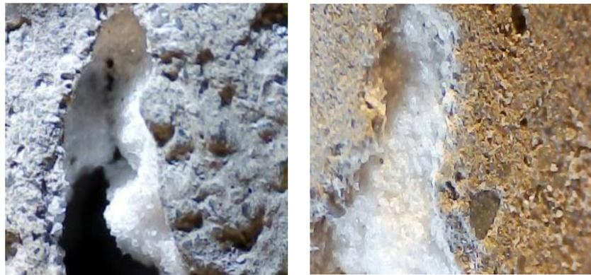
**Figure 11.** Sealed images of mortar cracks with 6% NC.
