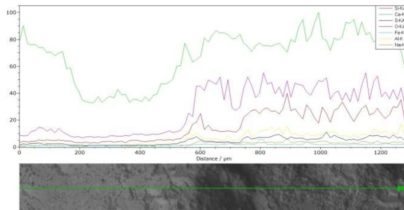
**Figure 8.** SEM images at 1200 magnifications and composition analysis.
