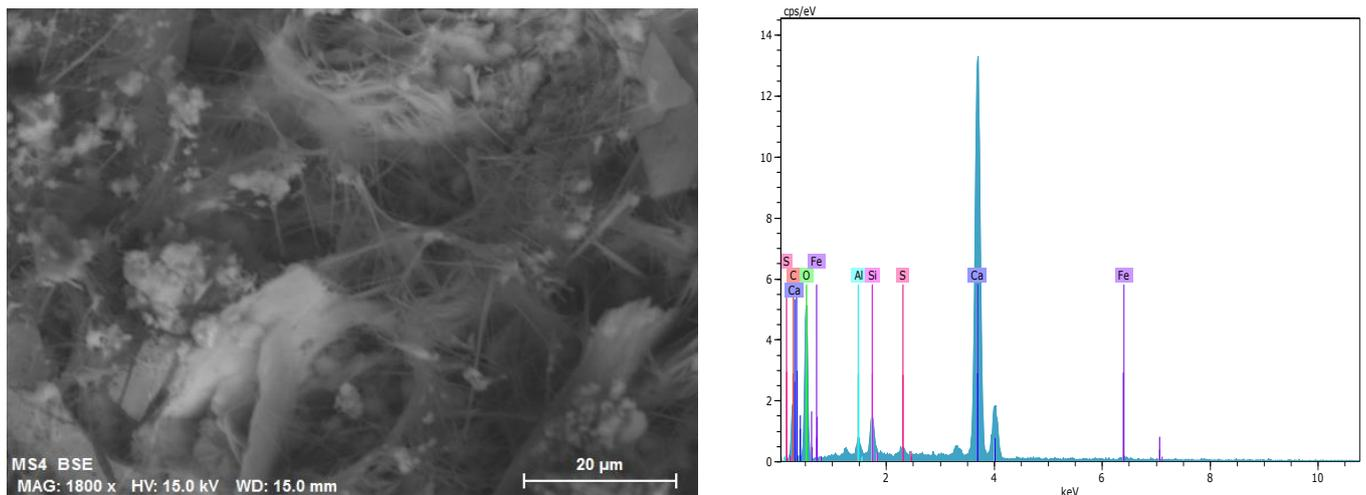
**Figure 9.** Microfissures filling with new ettringite-type hydration products.
