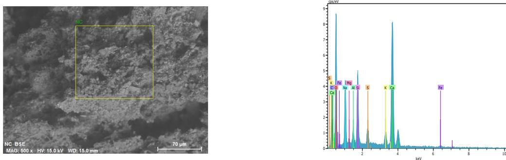
**Figure 6.** The chemical elements of EDS-tested healing products.
