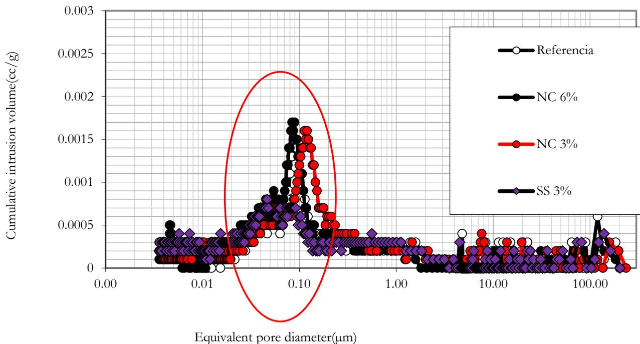
Figure 4. Mercury intrusion volume (cc/g).
