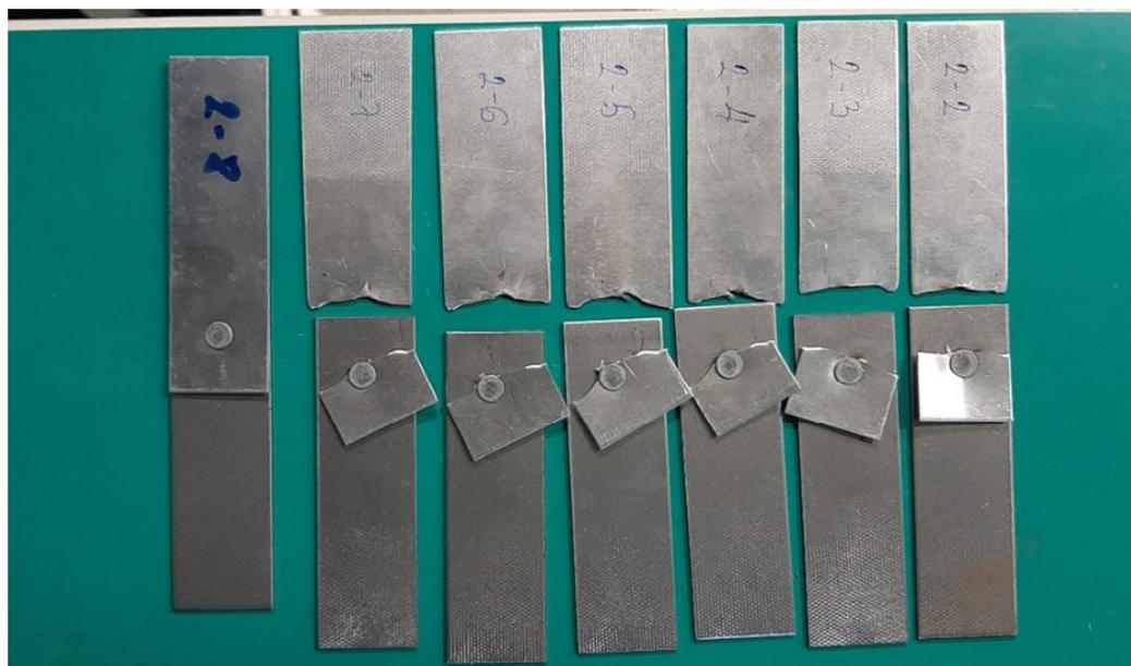
**Figure 10.** REW specimen fracture after dynamic tensile-shear testing.
