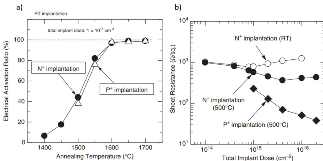
**Figure 10.** (a) Annealing-temperature dependence of the electrical activation ratio in nitrogen- (N) or phosphorus (P)-implanted SiC. (b) Sheet resistance versus the total implant dose for N- or P-implanted SiC annealed at 1700 °C for 30 min [125]. Copyright © 2022 John Wiley & Sons, Singapore Pte. Ltd.
