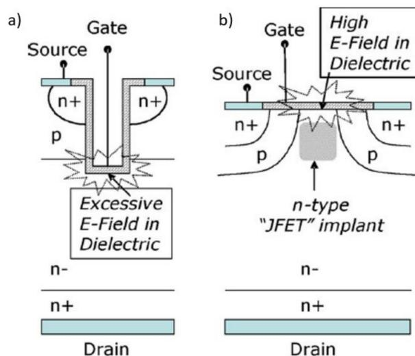
Figure 13. High electric field stress of (a) UMOFETs and (b) DMOSFETs [195].
