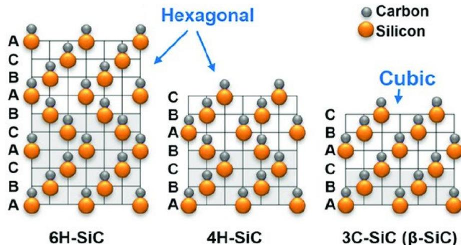
Figure 1. The stacking sequences of SiC polytypes: 4H-SiC, 6H-SiC, and 3C-SiC [16].
