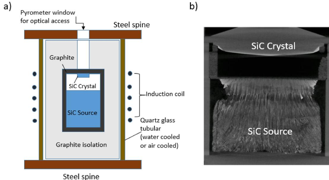
**Figure 6.** (a) A sketch of the PVT growth method for SiC boules and (b) 2D visualization of the PVT growth to image the great details about the morphology and the crystal growth interface and conditions [113].
