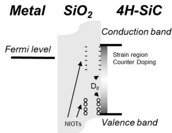
**Figure 11.** Graphical representation of the location of oxide traps and interface traps present at the interface of SiO<sub>2</sub>/4H-SiC [127].
