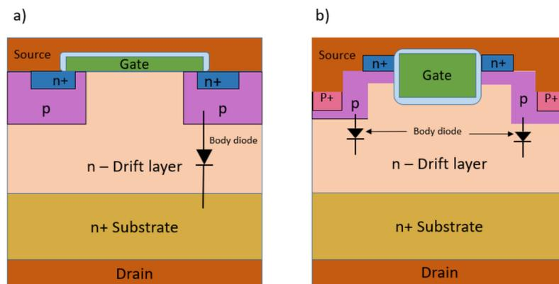
Figure 14. The location of body diode in (a) DMOSFETs and (b) UMOFETs.
