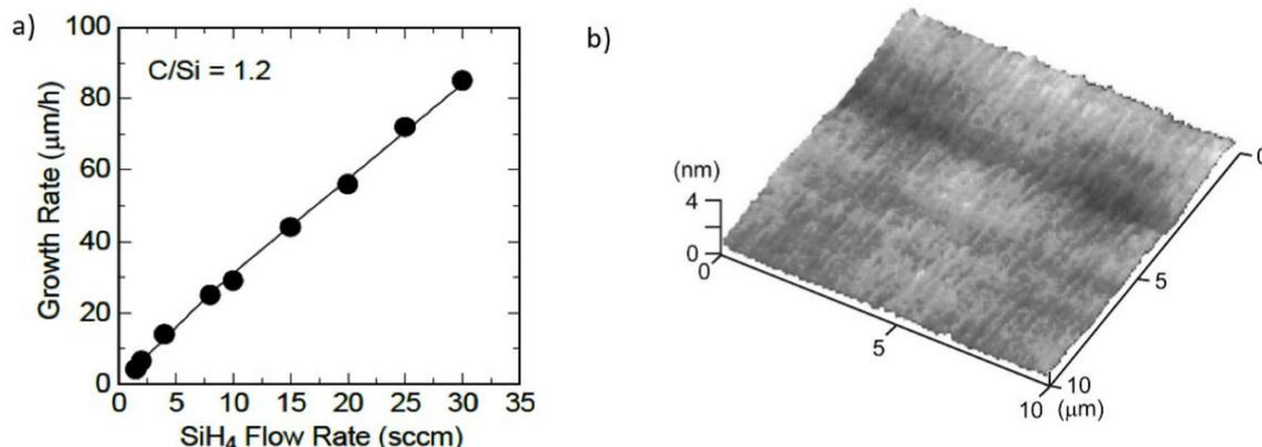
**Figure 8.** (a)  $\text{SiH}_4$ -flow-rate dependence of the growth rate at a C/Si ratio ( $\text{C/Si} = 1.2$ ) in the homoepitaxial growth of 4H-SiC(0001) [121,122]. (b) AFM results from a 150 mm-diameter 4H-SiC epitaxy grown at  $77\ \mu\text{m/h}$  [123].
