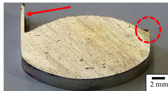
Figure 2. Formed oval cross-section of the magnesium wire pre-profile (AZ31); red markings indicate the burrs formed double-sided on the upper side of the wire.
