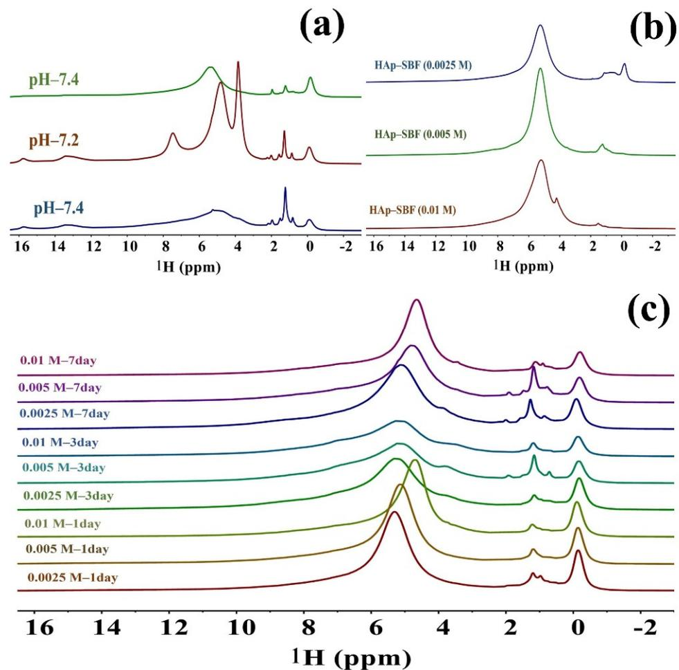
**Figure 3.** (a)  $^1\text{H}$  35 kHz MAS NMR spectra of HAp synthesized in different pH values; (b)  $^1\text{H}$  35 kHz MAS NMR spectra of F-HAp synthesized in BSF at different concentrations; (c)  $^1\text{H}$  35 kHz MAS NMR spectra of HAp soaked in NaF solutions with different concentrations and different times.
