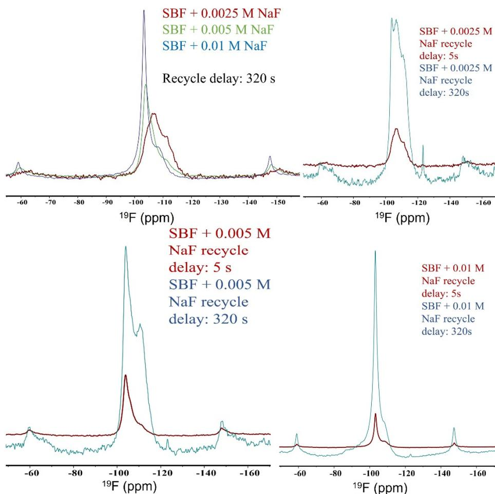
**Figure 4.**  $^{19}\text{F}$  35 kHz MAS spectra of HAp synthesized in SBF and soaked in solutions at different NaF concentrations (2.5 mM, 5 mM, and 10 mM) for different recycle delays (brown: 5 s; green: 320 s).
