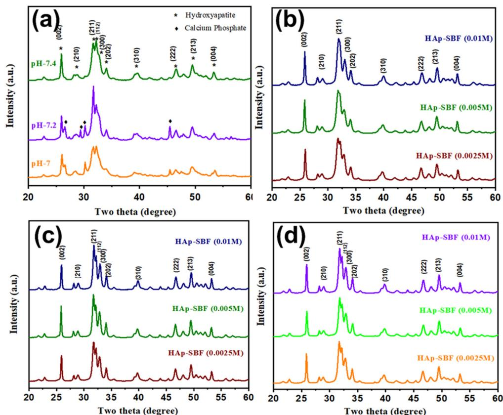
**Figure 1.** Powder XRD spectra of HAp and F-HAp (a): HAp synthesized in SBF at different pH values; (b): F-HAp synthesized in SBF at different concentrations of NaF; (c): HAp synthesized in SBF followed by 1 day soaking in solutions of different concentrations of NaF; (d): HAp synthesized in SBF followed by 3 days soaking in solutions of different concentrations of NaF.
