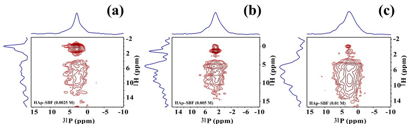
**Figure 5.**  $^1\text{H}$ - $^{31}\text{P}$  35 kHz HETCOR spectra of HAp synthesized in SBF and NaF solutions at different concentrations: 2.5 mM (a), 5 mM (b), and 10 mM (c).
