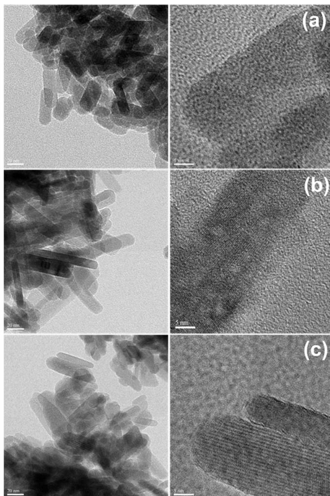
**Figure 2.** HRTEM images of F-HAp: (a) F-HAp synthesized in SBF at 0.01 M of NaF, (b) F-HAp synthesized in SBF at 0.005 M of NaF, and (c) F-HAp synthesized in SBF at 0.0025 M of NaF.
