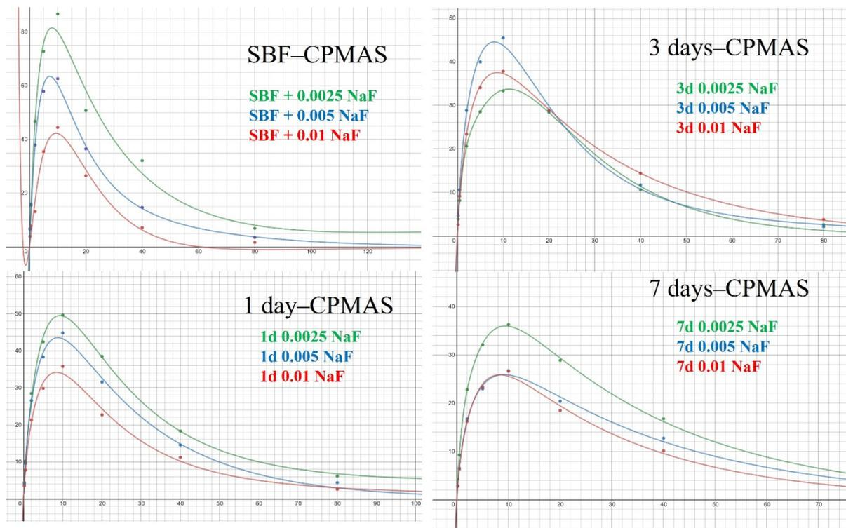
**Figure 7.**  $^1\text{H}$ - $^{31}\text{P}$  11 kHz CPMAS spectra of HAp synthesized in SBF and soaked in solutions at different NaF concentrations (2.5 mM, 5 mM, and 10 mM) for different recycle delays (brown: 5 s; green: 320 s).
