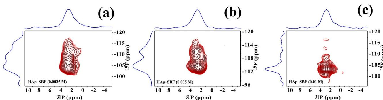
**Figure 6.**  $^{19}\text{F}$ - $^{31}\text{P}$  35 kHz HETCOR spectra of HAp synthesized in SBF and NaF solutions at different concentrations: 2.5 mM (a), 5 mM (b), and 10 mM (c). The gradual decrease of the cross peaks between  $\sim 108$  to  $\sim 114$  ppm corresponds to a decrease in the amorphous shell region and an increase of crystallinity.
