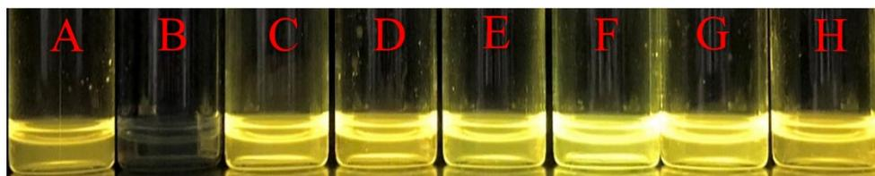
**Figure 12.** The color change resulting from combination of sensor R1 and different anions under UV lamp 365 nm, in order of (A) only sensor R1, (B) R1+F<sup>-</sup>, (C) R1+Cl<sup>-</sup>, (D) R1+Br<sup>-</sup>, (E) R1+CH<sub>3</sub>COO<sup>-</sup>, (F) R1+H<sub>2</sub>PO<sub>4</sub><sup>-</sup>, (G) R1+C<sub>6</sub>H<sub>5</sub>COO<sup>-</sup>, and (H) R1+I<sup>-</sup>.
