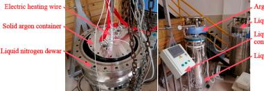
. Argon source . Liquid nitrogen source . Liquid nitrogen spraying controlling system . Liquid nitrogen dewar
