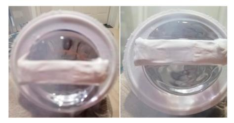
**Figure 7.** The white taped photodetector (MPPC with base board) coupled to the solid argon. The photodetector is put in the solid argon container before solid argon preparation.
