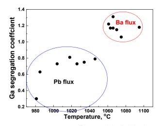
**Figure 3.** Ga segregation coefficients in (Tb,Al)<sub>3</sub>(Al,Ga)<sub>5</sub>O<sub>12</sub>:Ce SCFs deposited via the LPE method onto GAGG:Ce substrates, dependent on crystallization temperature.
