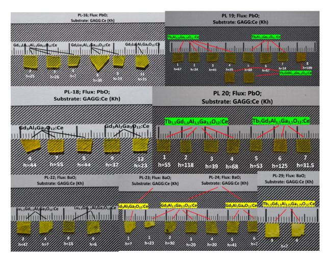
**Figure 1.** Multicomponent garnet composite scintillators fabricated in this work and their thicknesses in µm.
