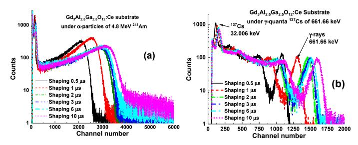
**Figure 7.** Pulse-height spectra of GAGG:Ce substrate under  $\alpha$ -particle (**a**) and  $\gamma$ -quantum (**b**) excitation measured at different shaping times.
