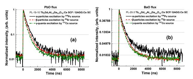
**Figure 11.** Scintillation decay of Tb<sub>2</sub>Gd<sub>1</sub>Al<sub>1.5</sub>Ga<sub>3.5</sub>O<sub>12</sub>:Ce SCF/GAGG:Ce SC (**a**) and Tb<sub>1.5</sub>Gd<sub>1.5</sub>Al<sub>1.5</sub> Ga<sub>3.5</sub>O<sub>12</sub>:Ce SCF/GAGG:Ce SC (**b**) composite scintillators grown from PbO- (**a**) and BaO-based fluxes, respectively, under  $\alpha$ - and  $\beta$ -particle and  $\gamma$ -ray excitations.
