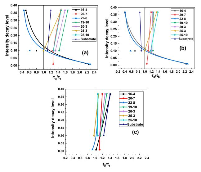
**Figure 10.**  $\tau_{\alpha}/\tau_{\gamma}$  (**a**),  $\tau_{a}/\tau_{\beta}$  (**b**), and  $\tau_{\beta}/\tau_{\gamma}$  (**c**) ratios of the selected multicomponent composite scintillators under study (see Table 4 for the sample denotations).
