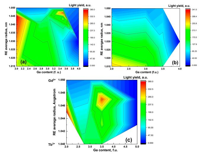
**Figure 4.** Light yield in  $(Gd,Lu,Tb)_3(Al,Ga)_5O_{12}$ : Ce films on GAGG: Ce substrates in dependence on average ionic radius of the rare earth ion and Ga content in the films under  $\alpha$ -particle excitation in (**a**) all the sample series, (**b**) Lu-Gd-substituted films, and (**c**) Gd-Tb-substituted films.
