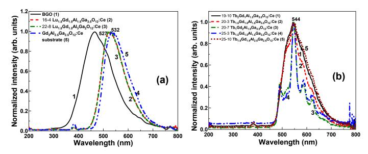
**Figure 6.** (a) Normalized XRL spectra of the selected Lu-Gd- (a) and Tb-Gd-based (b) composite scintillators in comparison with GAGG:Ce substrate and reference BGO scintillator.
