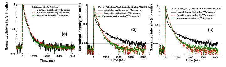
**Figure 9.** Scintillation decay of GAGG:Ce SC substrate (**a**) and Lu<sub>1.5</sub>Gd<sub>1.5</sub>Al<sub>1.5</sub>Ga<sub>3.5</sub>O<sub>12</sub>:Ce SCF/GAGG:Ce SC composite scintillators grown from PbO- (**b**) and BaO-based (**c**) fluxes under  $\alpha$ - and  $\beta$ -particle and  $\gamma$ -ray excitations.
