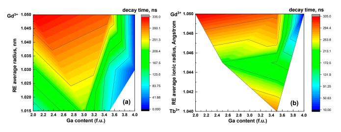
**Figure 5.** Scintillation decay time (1/e) in  $(Gd,Lu)_3(Al,Ga)_5O_{12}$ :Ce (**a**)  $(Gd,Tb)_3(Al,Ga)_5O_{12}$ :Ce (**b**) films in dependence on average ionic radius of the rare earth ion and Ga content in the films under  $\alpha$ -particle excitation.
