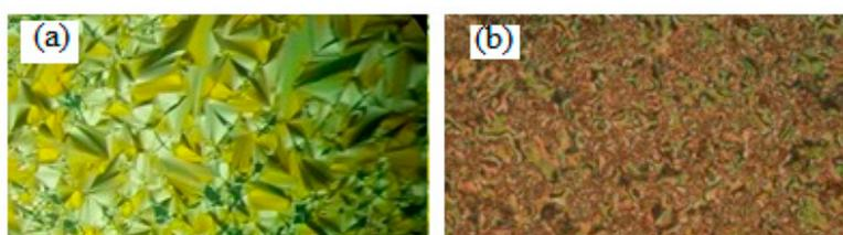
**Figure 4.** Smectic phases' textures upon cooling under POM for complex **Ic/II** (a) SmA phase at  $44.0\text{ }^{\circ}\text{C}$  and (b) SmC phase at  $25.0\text{ }^{\circ}\text{C}$ .
