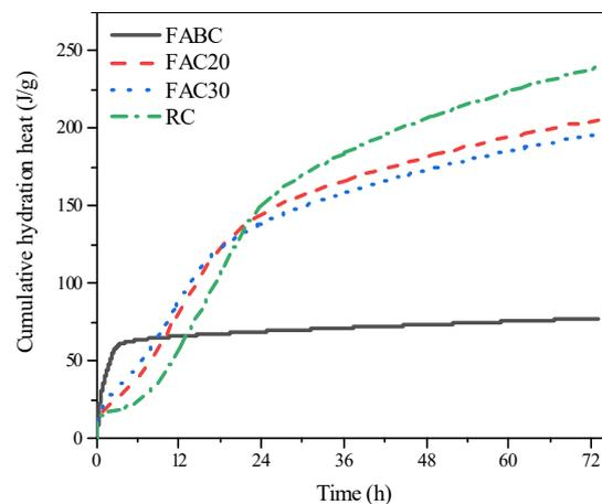
**Figure 2.** Hydration heat of cement with different FABC content.
