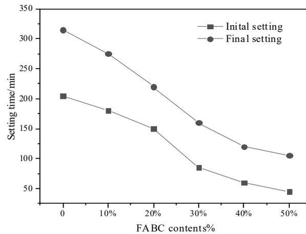
**Figure 1.** Setting time of cement with different FABC content.
