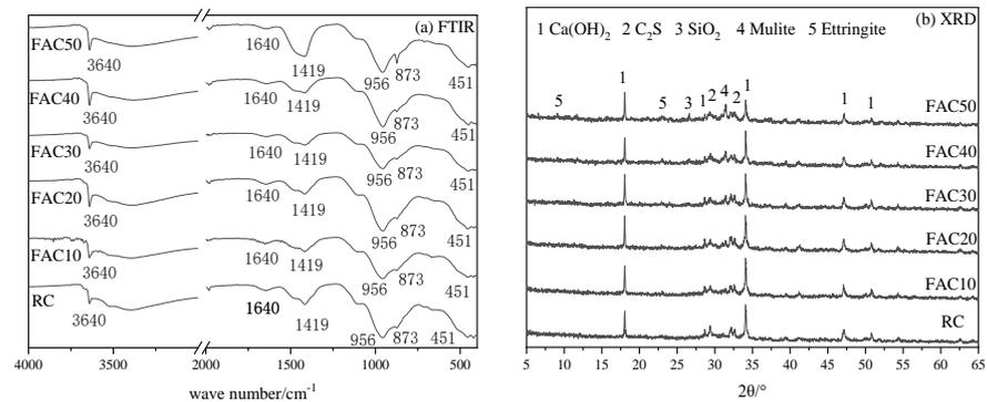
**Figure 5.** FTIR and XRD spectrum of pastes at 28 d: (a) FTIR; (b) XRD.
