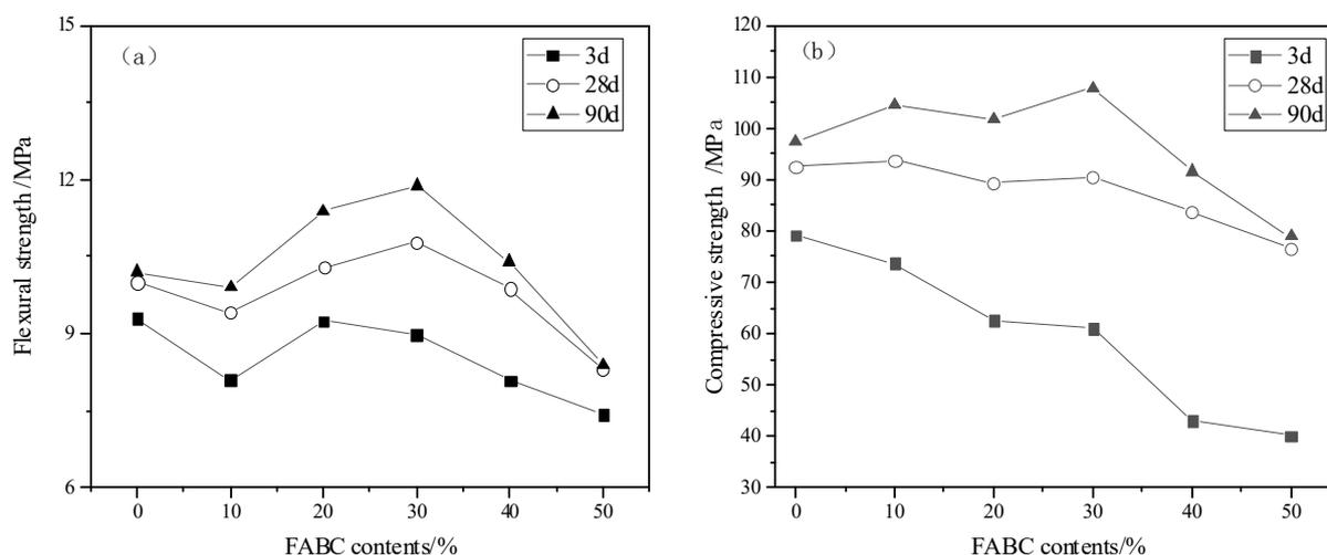
Figure 3. The strength of pastes with different FABC content: (a) Flexural strength; (b) Compressive strength.
