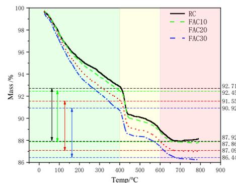
**Figure 6.** Thermal analysis of pastes at 3 d.
