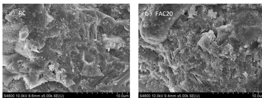
**Figure 7.** Micro-structure of Portland cement and composite cement pastes at 28d age: (a) RC; (b) FAC20.
