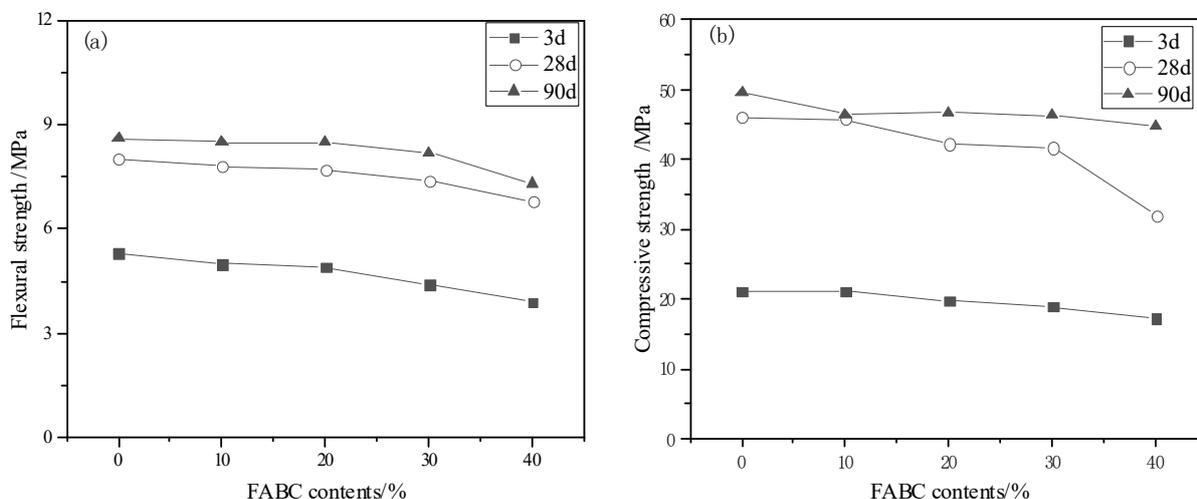
**Figure 4.** The strength of mortars with different FABC content: (a) Flexural strength; (b) Compressive strength.
