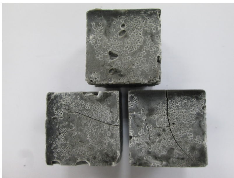
Figure 8. Thermal cracking in geopolymer specimens caused by overcuring.
