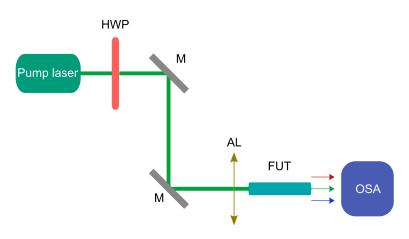
**Figure 8.** Experimental arrangement. Half-wave plate (HWP). Mirror (M). Aspherical lens (AL). Fiber under test (FUT). Optical spectrum analyzer (OSA).
