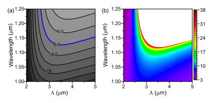
**Figure 4.** (a) Chromatic dispersion as a function of optical wavelength and fiber pitch for D<sub>2</sub>O-filled PCFs. Numbers indicates dispersion levels in ps/km·nm. (b) Frequency shift map of PMI–SF; color bars are detuning frequencies values in THz. Parameters used in the simulations:  $d/\Lambda = 0.56$ , P = 3 kW.
