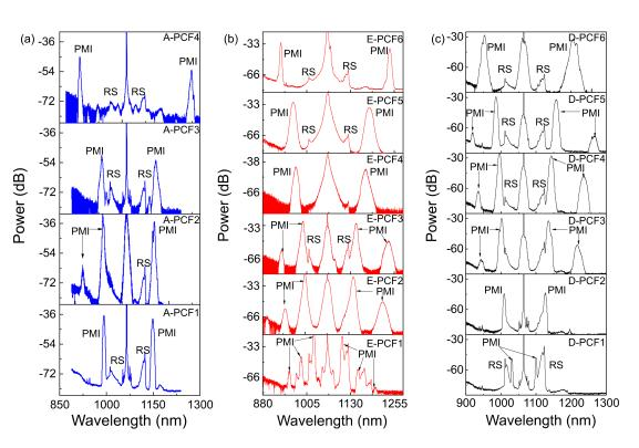
**Figure 10.** PMI spectra generated in (**a**) air-filled PCFs (blue line), (**b**) ethanol-filled PCFs (red line) and (**c**) D<sub>2</sub>O-filled PCFs (black line).
