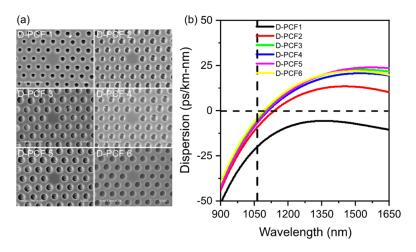
**Figure 7.** (a) SEM images of D<sub>2</sub>O-filled PCFs cross-section. (b) Chromatic dispersion of PCFs with holes filled with D<sub>2</sub>O. Dashed vertical black line indicates the experimental pump wavelength.
