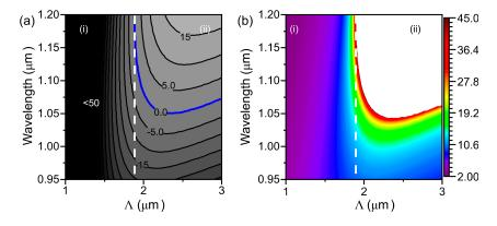
**Figure 2.** (a) Chromatic dispersion as a function of optical wavelength and fiber pitch for air-filled PCFs. Numbers indicates dispersion levels in ps/km·nm. White dashed line indicates pitch of 1.8  $\mu$ m. (b) Frequency shift map of polarization modulation instability (PMI–SF); color bars are detuning frequencies values in THz. Parameters used in the simulations:  $d/\Lambda = 0.36$ , P = 3 kW.
