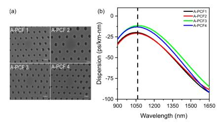
**Figure 5.** (a) SEM images of air-filled PCFs cross-section. (b) Chromatic dispersion of air-filled PCFs. Dashed vertical black line indicates the experimental pump wavelength.
