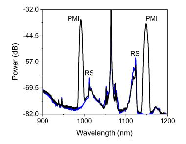
**Figure 9.** Light spectrum for two orthogonal polarization orientation of the pump. Pump polarization oriented to the fast axis (blue line) and to the slow axis (black line). Both spectra were recorded at pump peak power of 2.4 kW.
