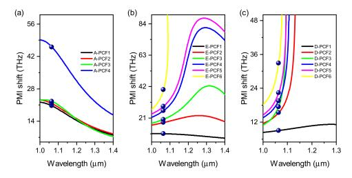
**Figure 11.** PMI–SF frequency shift as function of pump wavelength calculated for (**a**) air-filled PCFs, (**b**) ethanol-filled PCFs and (**c**) D<sub>2</sub>O-filled PCFs. Dots are experimental data. Peak power of 2.5 kW for air-filled PCFs and 3 kW for both ethanol-filled PCFs and D<sub>2</sub>O-filled PCFs.
