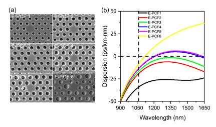
**Figure 6.** (**a**) SEM images of ethanol-filled PCFs cross-section. (**b**) Chromatic dispersion of PCFs with holes filled ethanol. Dashed vertical black line indicates the experimental pump wavelength.
