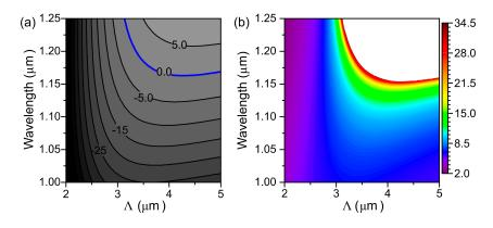
**Figure 3.** (a) Chromatic dispersion as a function of optical wavelength and fiber pitch for ethanolfilled PCFs. Numbers indicates dispersion levels in ps/km·nm. (b) Frequency shift map of PMI–SF; color bars are detuning frequencies values in THz. Parameters used in the simulations:  $d/\Lambda = 0.58$ , P = 3 kW.
