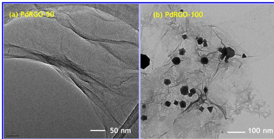
**Figure 4.** TEM images of green synthesized nanostructures: (a) RGO and (b) RGO-PN-100.
