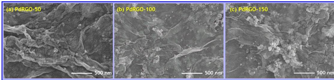
**Figure 3.** SEM micrographic images of green synthesized RGO-supported palladium nanoparticles with different concentrations: (a) RGO-PN-50, (b) RGO-PN-100, and (c) RGO-PN-150.
