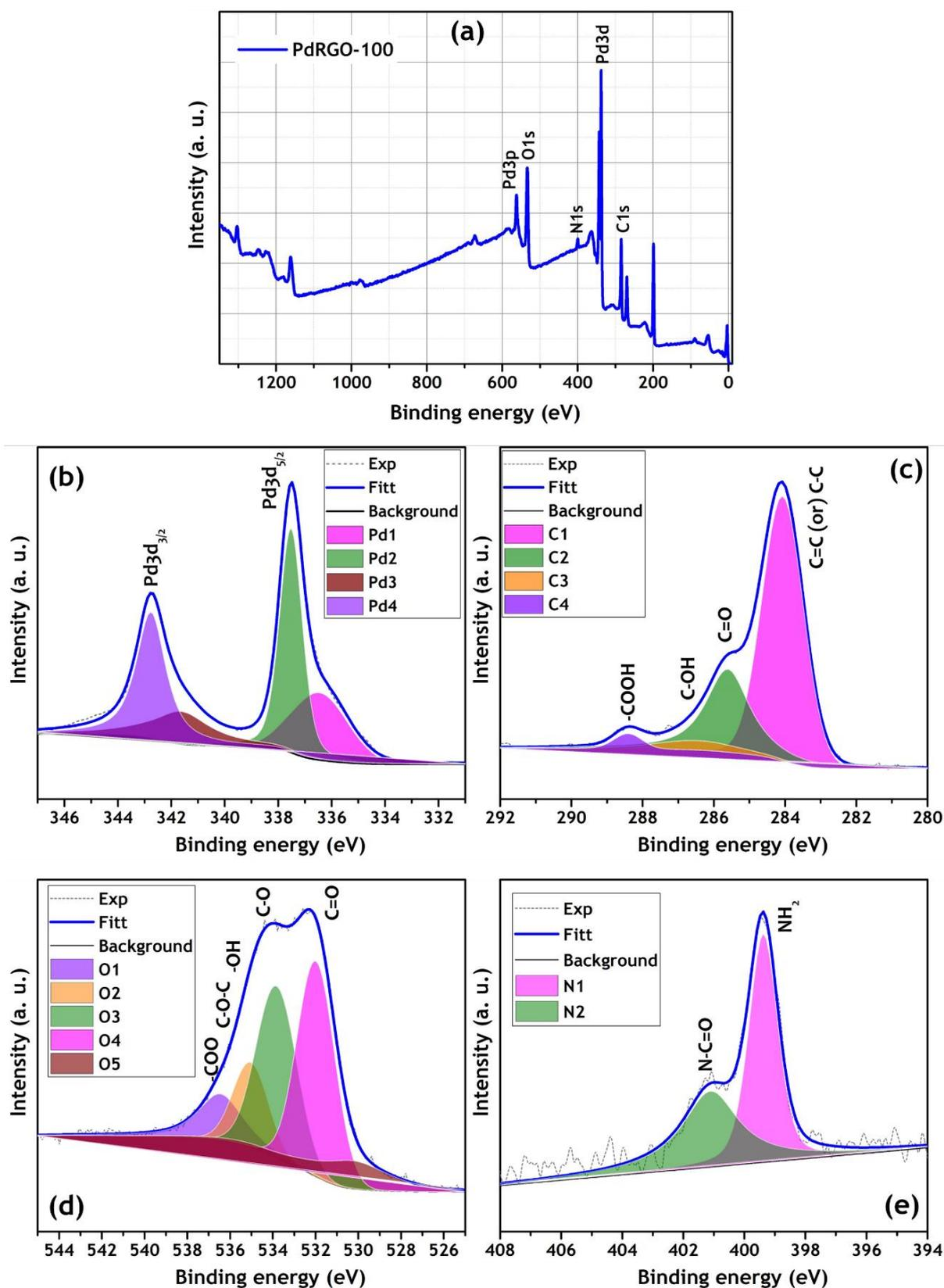
Figure 5. XPS spectra of RGO-PN100 for (a) survey scan, (b) palladium, (c) carbon, (d) oxygen, and (e) nitrogen elements.
