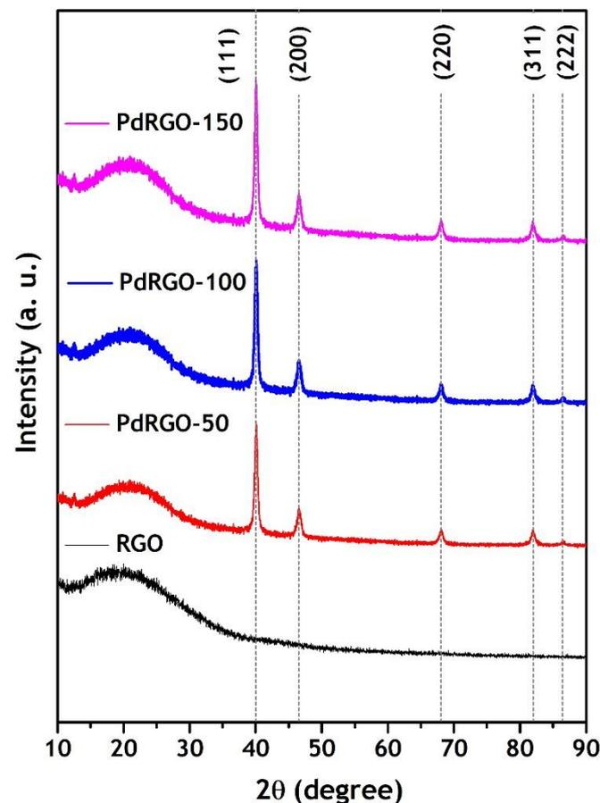
**Figure 2.** XRD patterns of RGO and green synthesized Pd-RGO nanoparticles from *Coleus amboinicus*.
