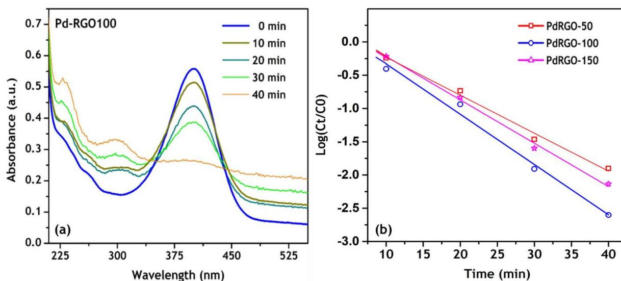
**Figure 6.** (a) Degradation kinetics of 4-nitrophenol using green synthesized RGO-PN100 from *Coleus amboinicus* (b) plots of reaction time versus  $\text{Log}(C_t/C_0)$ .
