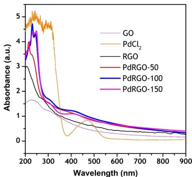
**Figure 1.** UV-Visible absorption pattern of graphene oxide (GO), PdCl<sub>2</sub>, reduced graphene oxide (RGO), and green synthesized palladium-reduced graphene oxide (Pd-RGO) nanoparticles from *Coleus amboinicus*.
