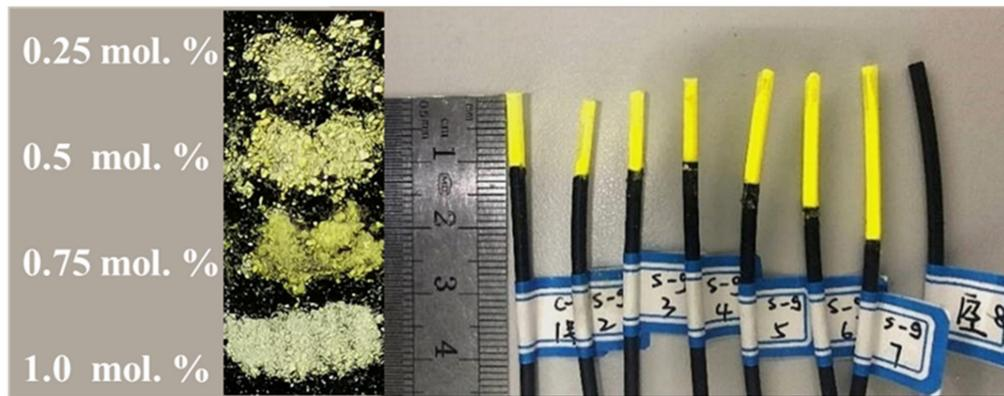
**Figure 1.** Eight YAG:Ce dosimeters with different parameters were made with the physical graph shown on the right side. On the left side are phosphors prepared via the sol-gel method; the color deepened as the concentration of Ce became higher; from top to bottom are YAG:Ce powders with Ce concentration of 0.25 mol.%, 0.5 mol.%, 0.75 mol.%, and 1 mol.%.
