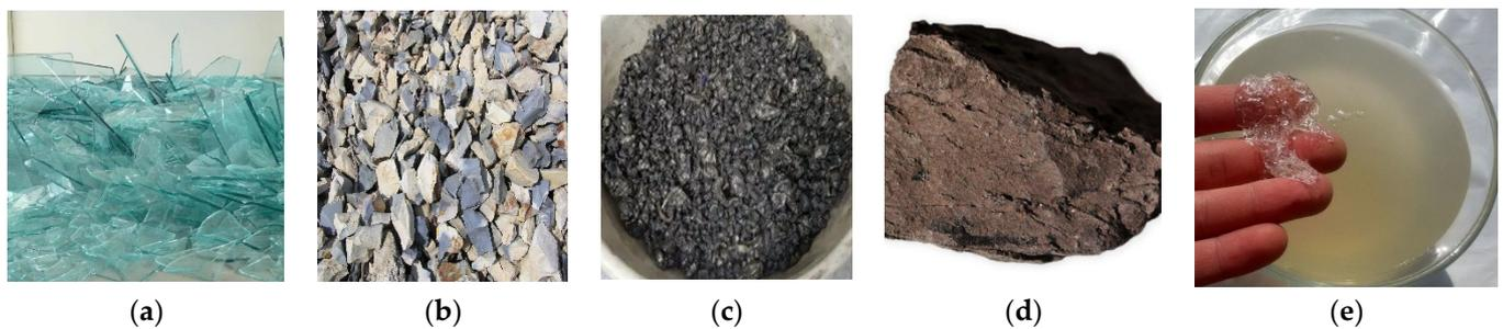
**Figure 1.** Appearance of the raw materials used: (a) glass breakage, (b) opoka, (c) WMS, (d) lignite clay, (e) liquid glass.
