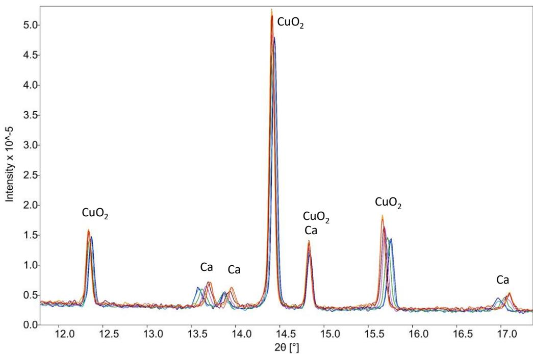
**Figure S3.** Synchrotron diffraction patterns collected from 320K to 950K (cold colors-lower temperature; warm colors-high temperature). The reflections associated to the Ca sub-structure manifest a progressive shift towards higher 2θ angles indicating the unusual shrinking of the lattice volume as the temperature increases. The CuO<sub>2</sub> sub-lattice shows the expected opposite trend.
