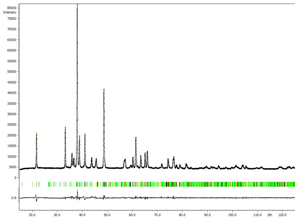
**Figure S2.** Rietveld plot obtained from the structural refinement of the (3D+1)-dimensional structure of composite crystal  $\text{Ca}_{0.83}\text{CuO}_2$  on PXRD data collected at RT.
