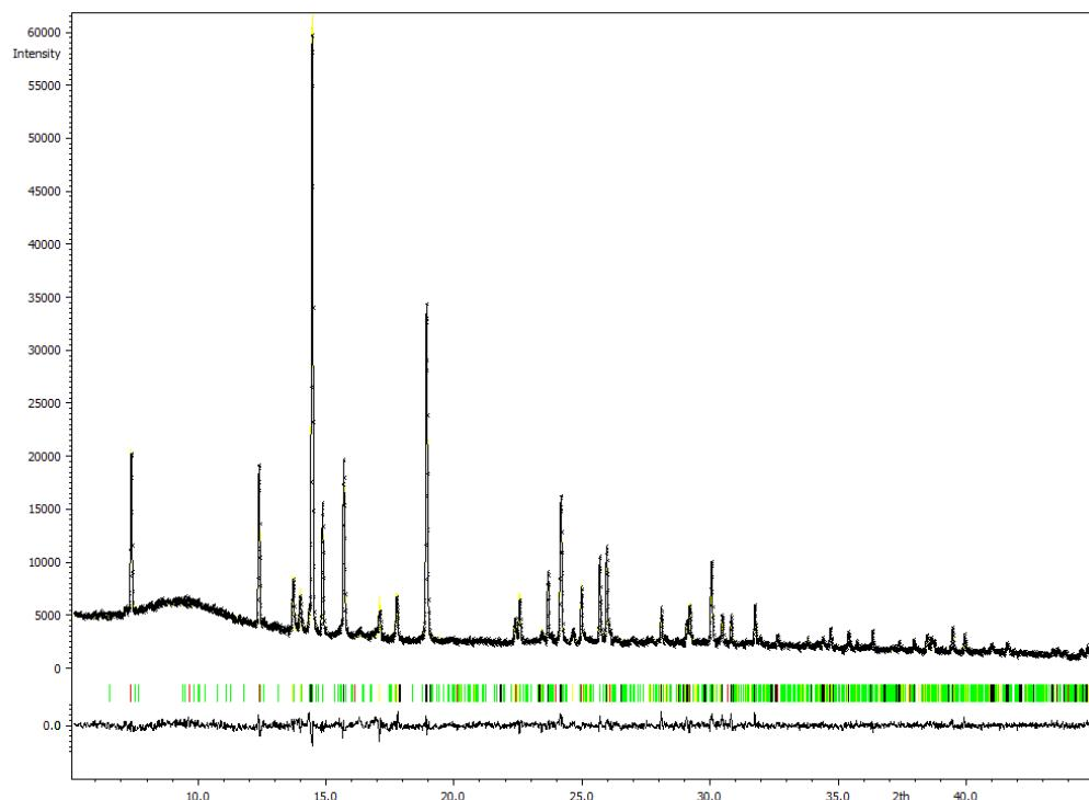
**Figure S4.** Rietveld plot obtained from the structural refinement of the Ca-based composite crystal on synchrotron diffraction data ( $\lambda=0.685\text{\AA}$ ) collected at 890K. The bump observed at around  $10^\circ$  of  $2\theta$  is related to the contribution of the glass tube containing the sample.
