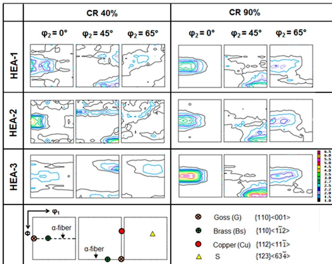
**Figure 5.** Texture of cold-rolled (CR) HEAs 1–3 represented by  $\phi_2 = 0^\circ, 45^\circ,$  and  $65^\circ$  orientation distribution function (ODF) sections (intensities are given in multiples of a random distribution). Lower ODF sections give the position of the typical rolling components of face-centered cubic (FCC) metals and alloys.
