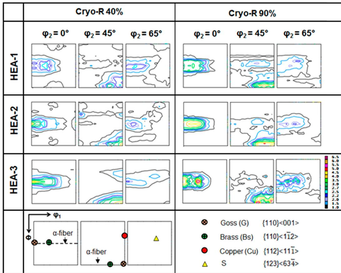
**Figure 6.** Texture of cryo-rolled (Cryo-R) HEAs 1–3 represented by  $\varphi_2 = 0^\circ, 45^\circ,$  and  $65^\circ$  ODF sections (intensities are given in multiples of a random distribution). Lower ODF sections give the position of the typical rolling components of FCC metals and alloys.
