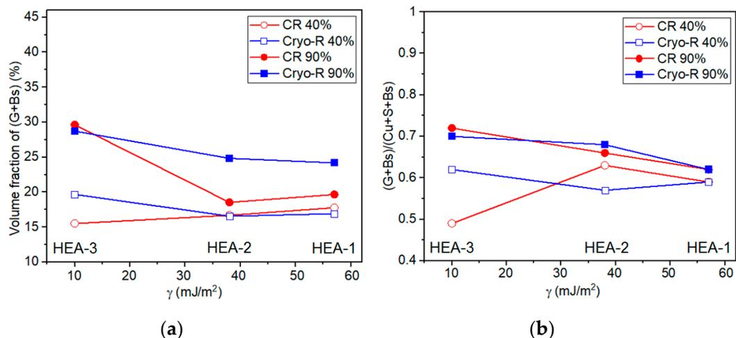
**Figure 8.** (a) Volume fraction of the  $\alpha$ -fiber components (G + B<sub>s</sub>) and (b) the ratio of the volume fractions of the  $\alpha$ -fiber (G + B<sub>s</sub>) and  $\beta$ -fiber components (Cu + S + B<sub>s</sub>) as a function of the stacking fault energy  $\gamma$ .
