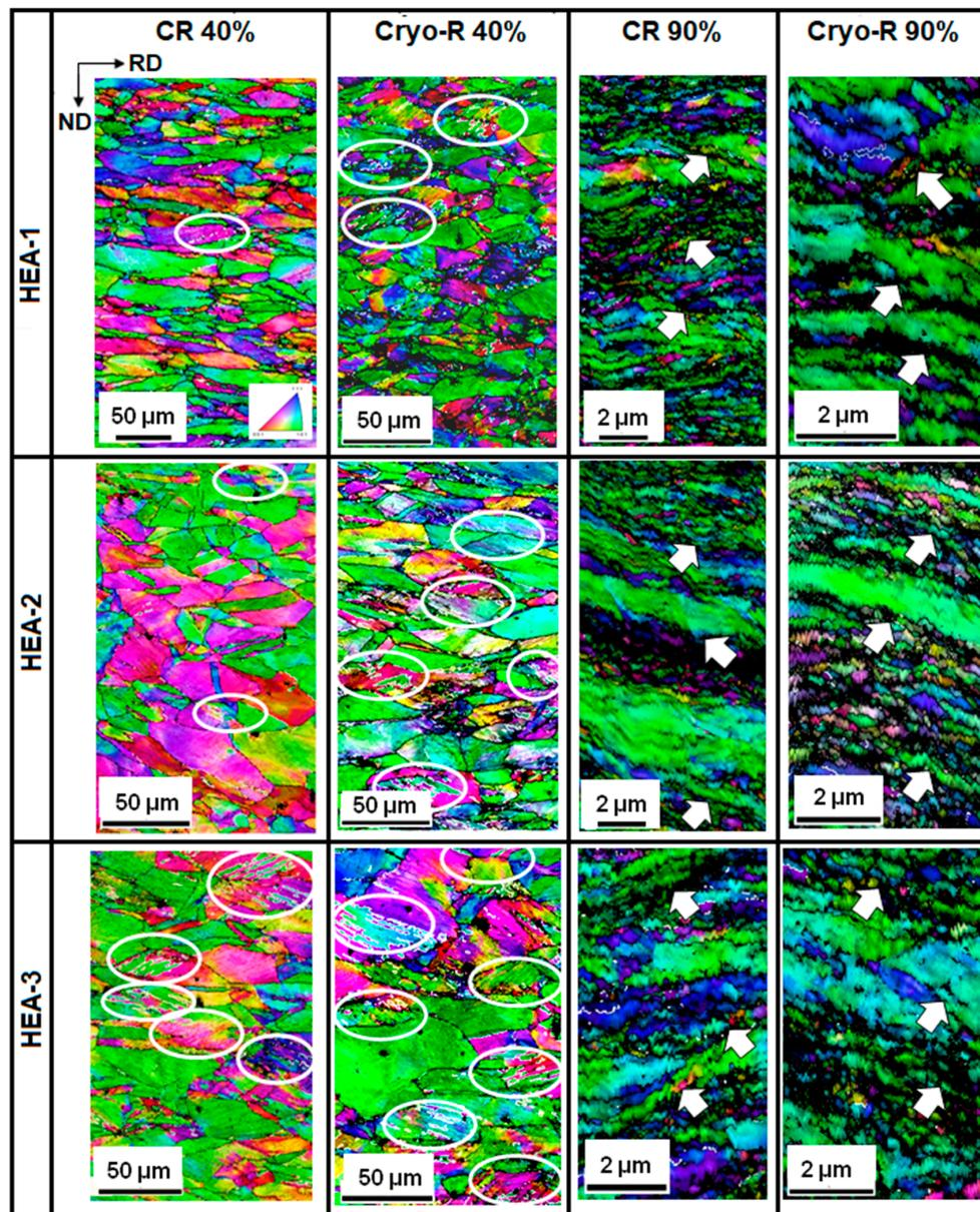
**Figure 3.** Microstructure of cold-rolled (CR) and cryo-rolled (Cryo-R) HEAs 1–3 represented by IPF maps (black lines: high angle grain boundaries; white lines:  $\Sigma 3$  twin boundaries (bundles marked by ellipses); fine-scale shear bands marked by arrows; color coding of the normal direction).
