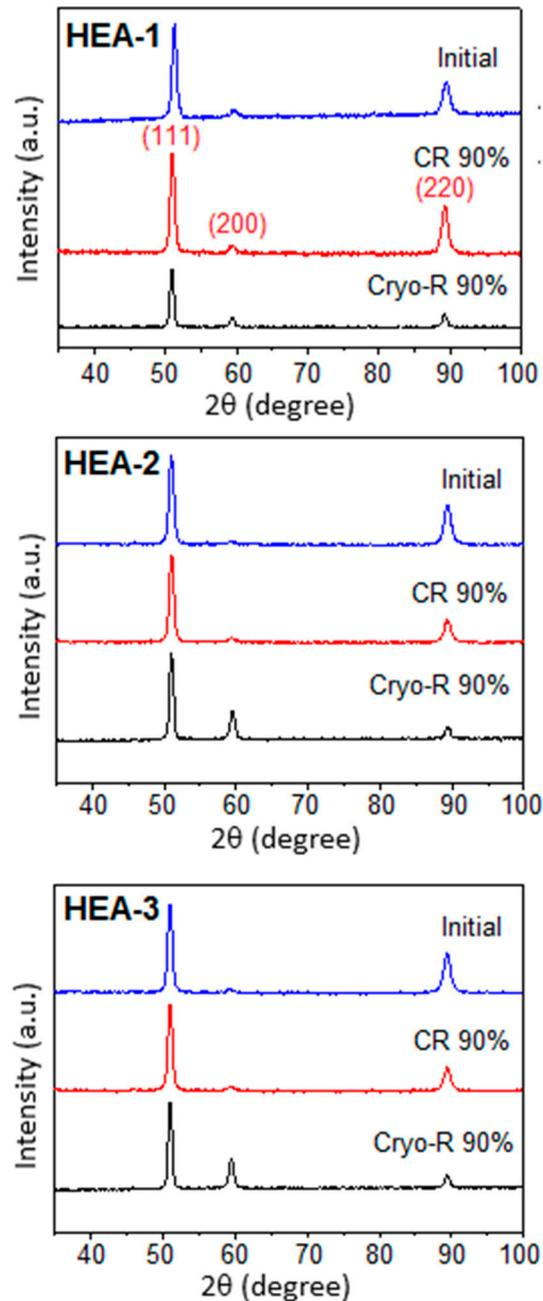
**Figure 1.** X-ray diffractograms of high-entropy alloys (HEAs) 1–3 before (initial) and after the 90% rolling reduction at room temperature (CR 90%) and cryogenic temperature (Cryo-R 90%).
