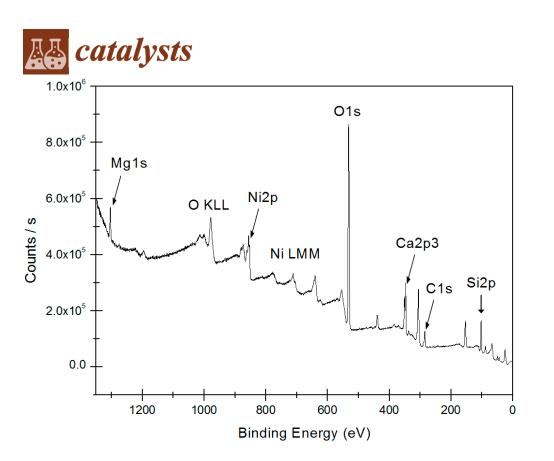
Figure 1S. XPS wide scan spectrum of the reduced Ni/ATP catalyst
