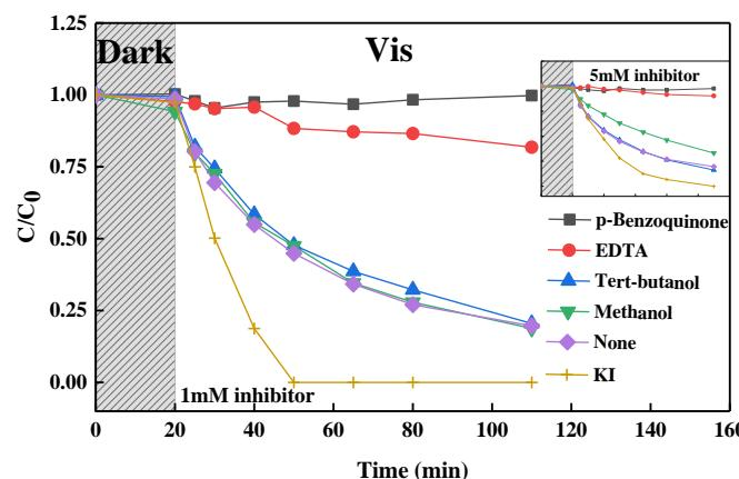
**Figure 9.** The relationship between  $\text{C}/\text{C}_0$  and  $t$  of the effect of the inhibitor on the photocatalytic activity of rGO–P25 photocatalyst. (visible wavelength 420 nm, 10 tubes, catalyst concentration 0.5 g/L, initial concentration of BPA 0.01 mol/mL, inhibitor concentration is 1 mol/mL, solution volume is 100 mL).
