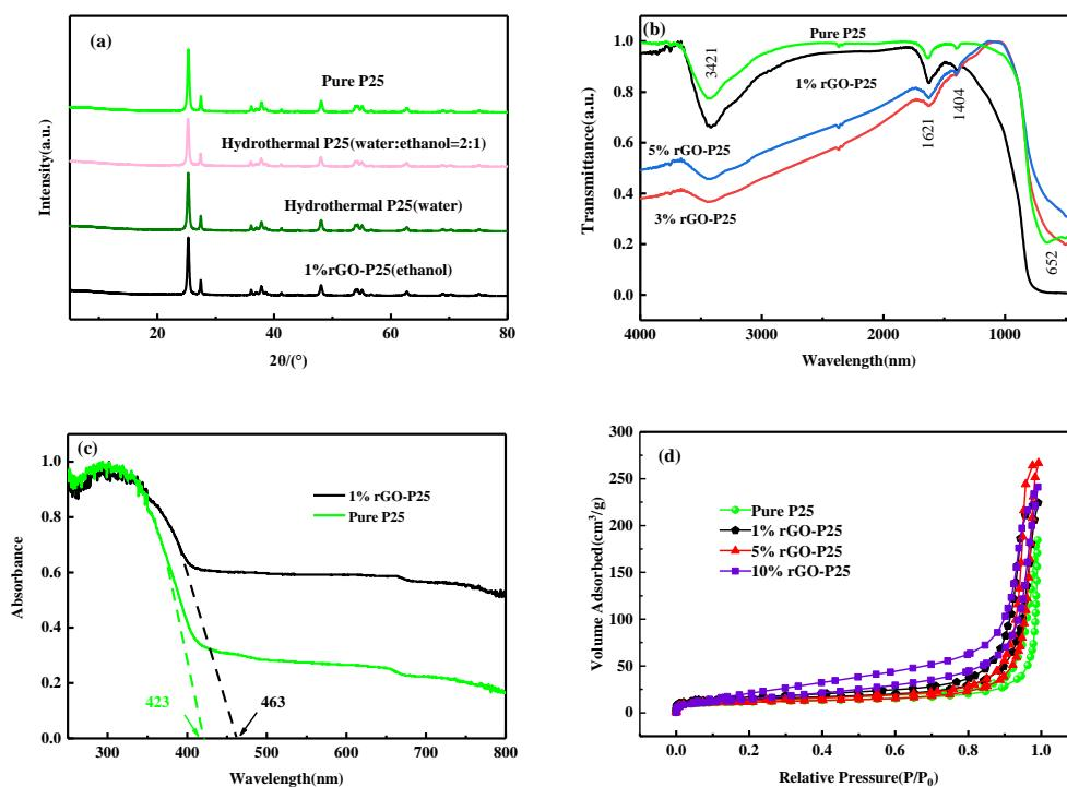
**Figure 2.** (a) XRD patterns of 4 photocatalysts; (b) FTIR spectra of pure P25, 1%, 3%, and 5% rGO-P25; (c) UV-vis diffuse reflectance spectra of pure P25 and 1% rGO-P25; (d) Nitrogen adsorption-desorption isotherms of P25, 1%, 5%, and 10% rGO-P25.
