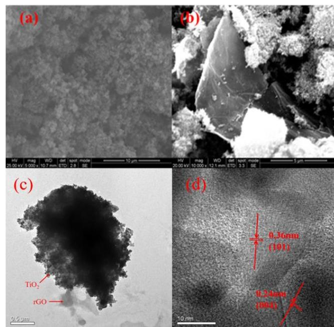
**Figure 1.** Scanning Electron Microscope (SEM) images of (a) pure P25; (b) 1% reduced graphene oxide-titanium dioxide photocatalyst ( $\text{rGO}-\text{TiO}_2$ ) composite photocatalyst with ethanol as solvent; (c) TEM micrographs of 1% rGO-P25 and (d) HRTEM image of 1% rGO-P25.
