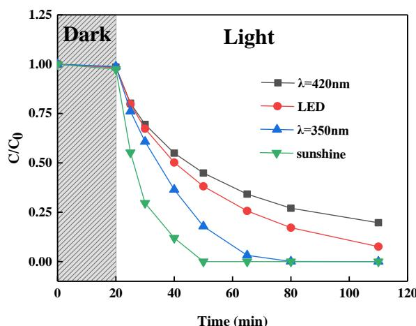
**Figure 7.** The relationship between  $C/C_0$  and  $t$  of the effect of different light sources on the photocatalytic activity of 1% rGO–P25 photocatalyst (catalyst concentration 0.5 g/L, the initial concentration of BPA is 0.01 mol/mL, solution volume is 100 mL).
