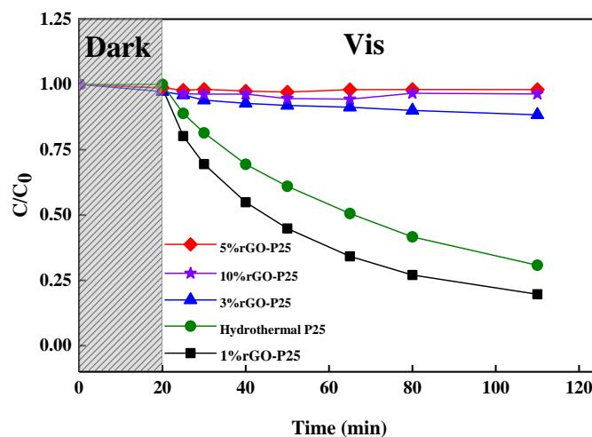
**Figure 4.** Effect of contents of rGO on BPA degradation by rGO-P25 under visible light irradiation (BPA concentration = 0.01 mol/L, catalyst dosage = 0.5 g/L, volume of the solution = 100 mL,  $\lambda$  = 420 nm, 10 tubes).
