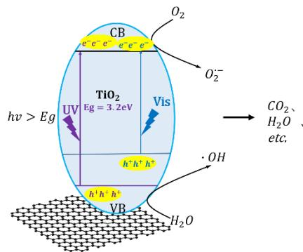
**Figure 8.** Photocatalytic reaction mechanism.
