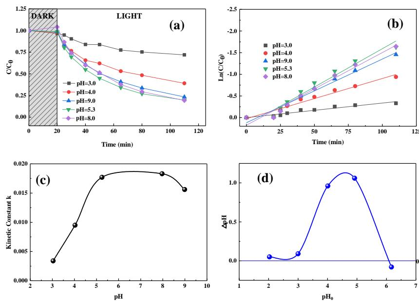
**Figure 6.** Effect of solution pH on BPA degradation under visible light irradiation. (a) curve of  $C/C_0$  versus time; (b) corresponding  $\ln(C/C_0)$  and time curve; (c) first-order kinetic curve of  $k$  versus catalyst concentration (BPA concentration = 0.01 mol/L, catalyst dosage = 0.5 g/L, volume of the solution = 100 mL,  $\lambda$  = 420 nm, 10 tubes); and (d) isoelectric point of 1% rGO–P25 composite photocatalyst.
