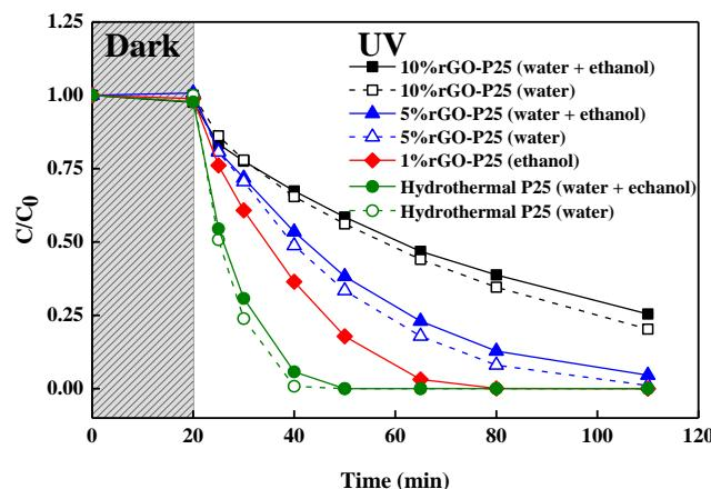
**Figure 3.** Effect of solvents and contents of rGO on bisphenol A (BPA) degradation by rGO-P25 under UV-light irradiation (BPA concentration = 0.01 mol/L, catalyst dosage = 0.5 g/L, volume of the solution = 100 mL,  $\lambda$  = 350 nm, ten tubes).
