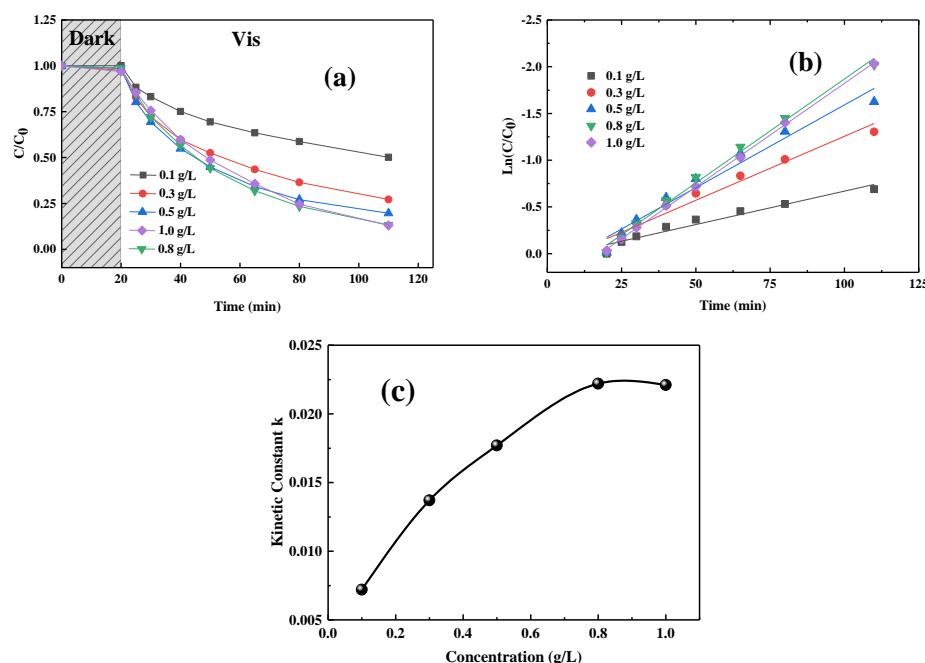
**Figure 5.** Effect of the concentration of 1% rGO-P25 on BPA degradation under visible light irradiation.
