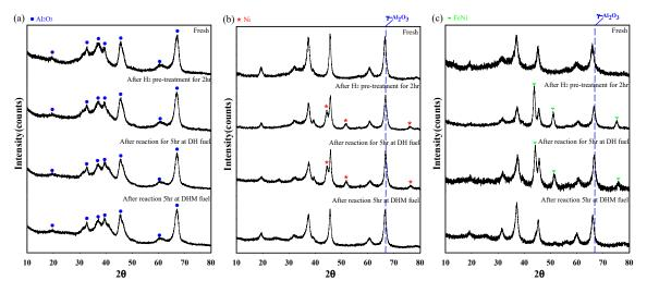
Figure 4. Results of XRD analysis performed on (a) R5A-I, (b) N10A, and (c) F10N10.
