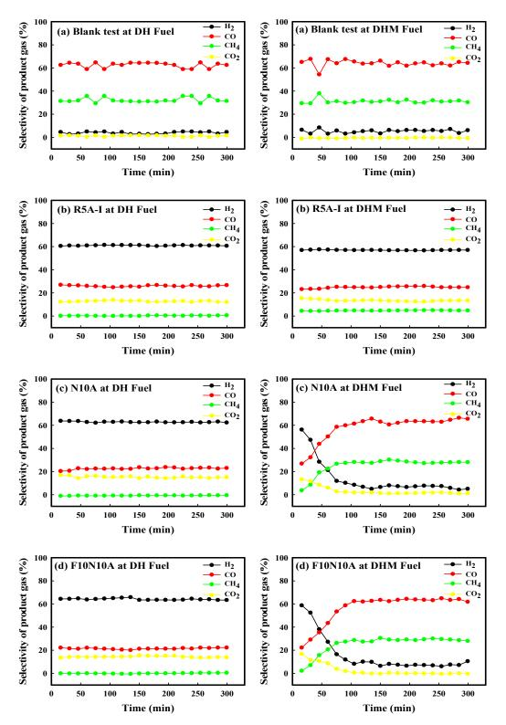
**Figure 2.** The selectivity of product gas (%) of the (a) blank test, (b) R5A-I, (c) N10A, and (d) F10N10A at DH and DHM fuel.
