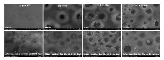
Figure 7. Scanning electron micrographs of (a) R5A-I, (b) N50A, (c) R1N50A, and (d) R2N50A.
