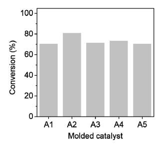
**Figure S2.** Ethanol conversion obtained after 3 h on steam in dehydration of bioethanol over 2 g of molded H-ZSM-5A1, H-ZSM-5A2, H-ZSM-5A3, H-ZSM-5A4, and H-ZSM-5A5 catalysts at  $250~^{\circ}$ C and  $5~h^{-1}$  WHSV.
