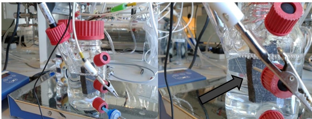
Figure S1. Experimental setup for H 2 measurement in close proximity to the cathode surface of a MES reactor. As indicated by the black arrow, the tip of a H 2 microsensor was positioned close to the surface of the cathode of a MES reactor to measure H 2 concentration at this specific location.
