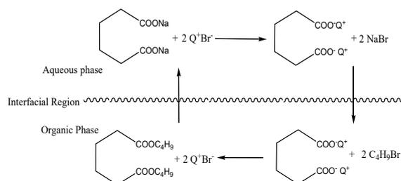
**Figure 10.** Esterification process by PTC.
