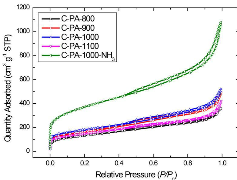
**Figure 1.** Nitrogen sorption isotherms of the synthesized carbon materials (STP: standard temperature and pressure).
