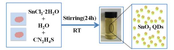
Figure 2. Colloidal synthesis of SnO<sub>2</sub> QDs [35], Copyright 2020, ACS.
