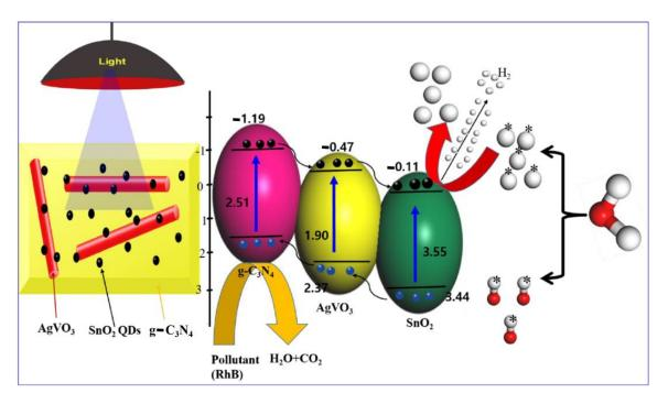
**Figure 7.** Photocatalytic mechanism of the ternary photocatalyst (SnO<sub>2</sub>/AgVO<sub>3</sub>/g-C<sub>3</sub>N<sub>4</sub>) [24], Copyright 2019, Springer.
