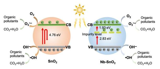
**Figure 4.** Photocatalytic mechanism of pure SnO<sub>2</sub> QDs and Nb-SnO<sub>2</sub> QDs [45], Copyright 2022, Elsevier.
