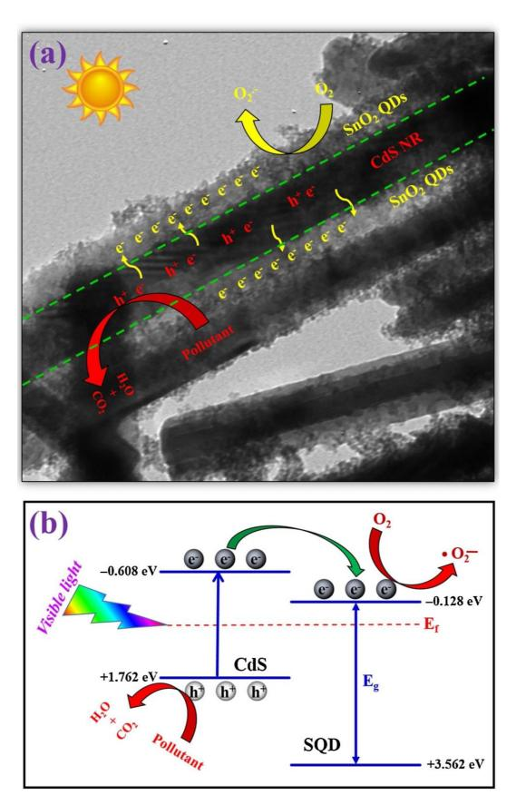
**Figure 5.** (a) CdS@SnO<sub>2</sub> core-shell NRs' photocatalytic degradation and (b) charge-transfer mechanism [40], Copyright 2019, Elsevier.
