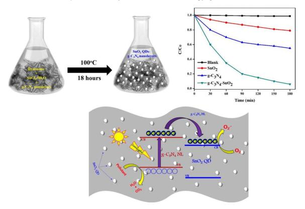
Figure 3. Synthesis and photocatalytic application of SnO<sub>2</sub> QDs [41], Copyright 2018, Elsevier.
