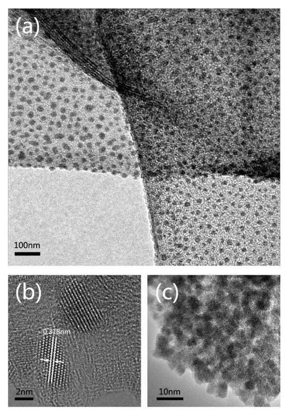
Figure 6. TEM images of SnO<sub>2</sub> QDs/rGO (**a**,**b**), pure SnO<sub>2</sub> QDs (**c**) [71], Copyright 2019, Elsevier.
