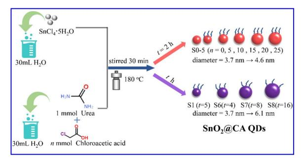
**Figure 1.** Diagrammatic representation of the SnO<sub>2</sub> QD synthesis process [34], Copyright 2021, Elsevier.
