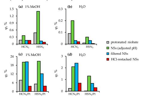
**Figure 8.** Comparison of apparent quantum efficiency of hydrogen generation from 1 mol.% aqueous methanol and water over the protonated niobates and their nanosheet-based photocatalysts in a bare state (**a**,**b**) and after surface platinization (**c**,**d**).
