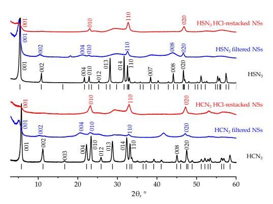
Figure 1. Powder XRD patterns of the protonated niobates and their reassembled nanosheets.
