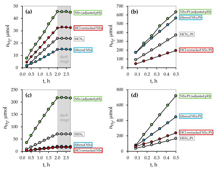
**Figure 7.** Kinetic curves of photocatalytic hydrogen evolution from 1 mol.% aqueous methanol over the HCN<sub>3</sub> (**a**,**b**) and HSN<sub>3</sub> (**c**,**d**) protonated niobates and their nanosheet-based photocatalysts.
