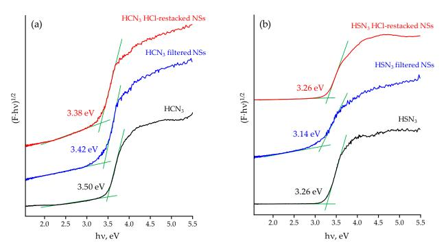
**Figure 3.** Tauc plots for the protonated forms and reassembled nanosheets of HCN<sub>3</sub> (**a**) and HSN<sub>3</sub> (**b**) niobates.
