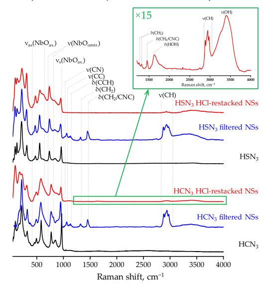
Figure 2. Raman spectra of the protonated niobates and their reassembled nanosheets.
