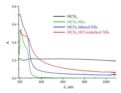
**Figure 6.** Typical UV-vis spectra of the suspensions of HCN<sub>3</sub>, its pristine as well as reassembled and redispersed nanosheets.
