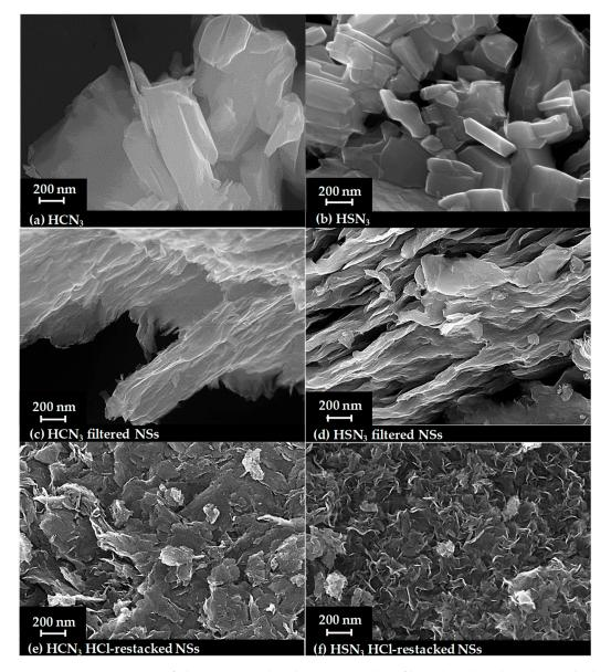
Figure 5. SEM images of the protonated niobates (**a**,**b**), their filtered (**c**,**d**) and HCl-restacked nanosheets (**e**,**f**).
