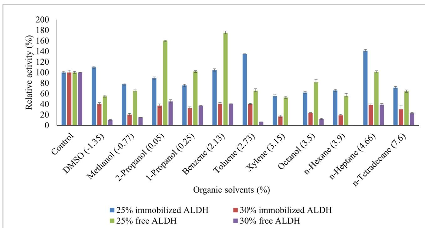
**Figure 6.** Comparison of effect of organic solvents on the stability of immobilized ALDH and free ALDH. Blue bar: 25% *v/v* immobilized ALDH; red bar: 30% *v/v* immobilized ALDH; green bar: 25% *v/v* free ALDH; purple bar: 30% *v/v* free ALDH. Each point represents the mean of three experiments  $\pm$  S.E. The value in the bracket represents the log *p*-value of the organic solvents.
