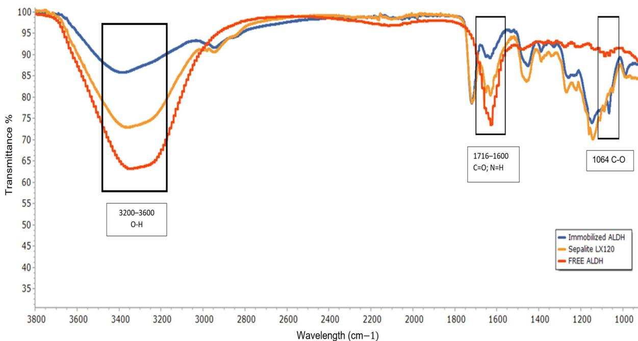
**Figure 2.** FTIR spectra of empty Seplite LX120, immobilized and free ALDH. Blue line: immobilized ALDH; orange line: empty Seplite LX120; red line: free ALDH.
