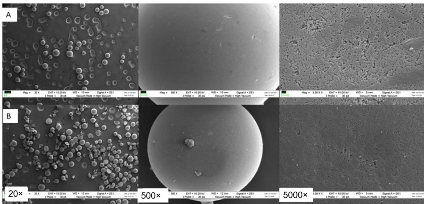
**Figure 3.** Scanning electron microscopy images of (A) empty Seplite LX120 and (B) immobilized ALDH. The images were captured at magnifications 20 $\times$ , 500 $\times$  and 5000 $\times$ .
