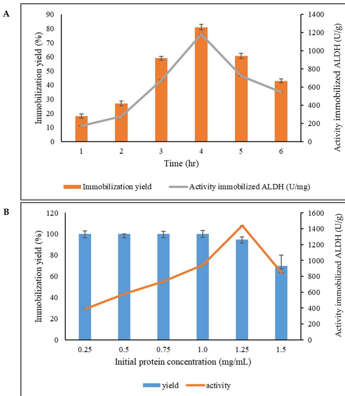
**Figure 1.** Optimization condition of the purified ALDH immobilized onto Seplite LX120. **(A):** The effect of immobilization time for the purified ALDH. **(B):** The effect of enzyme loading for ALDH immobilization. The bar chart shows the immobilization yield (%) for the ALDH. The line graph indicates the activity (U/mg) of the immobilized ALDH. Each point represents the mean of three experiments  $\pm$  S.E.
