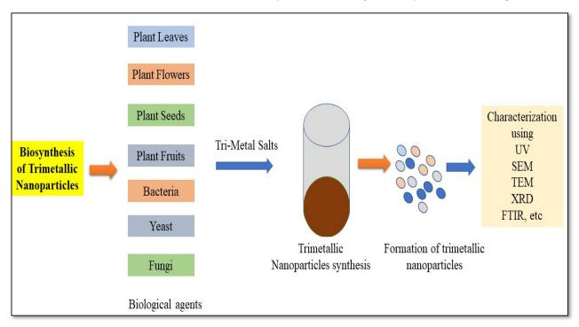
Figure 3. Biological synthesis of trimetallic nanoparticles.
