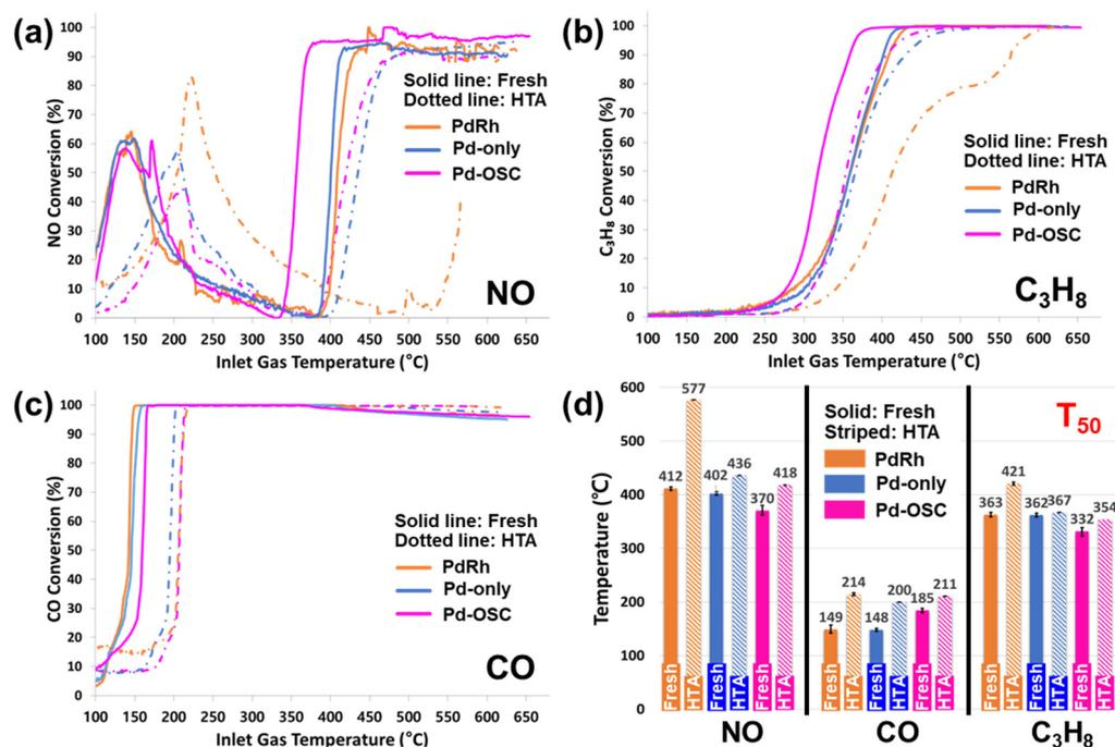
**Figure 2.** Effect of inlet gas temperature on the conversion of (a) NO, (b) C<sub>3</sub>H<sub>8</sub>, and (c) CO and (d) T<sub>50</sub> of each gas species for PdRh, Pd-only, and Pd-OSC fresh and HTA samples at stoichiometric condition.
