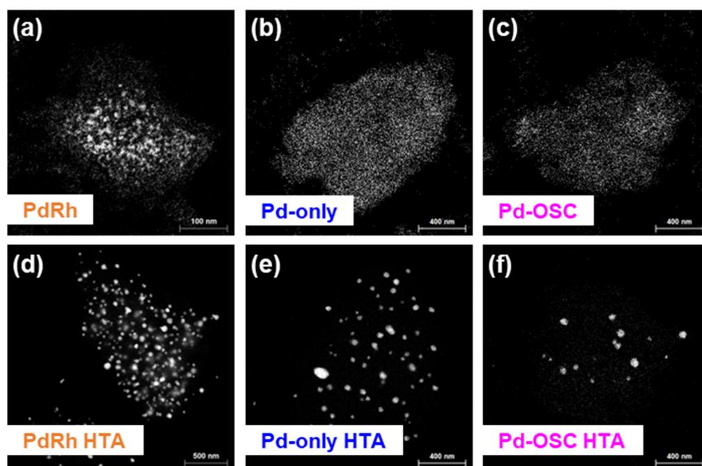
**Figure 6.** STEM images of Pd particles for PdRh, Pd-only, and Pd-OSC TWC fresh (a–c) and HTA (d–f) samples.
