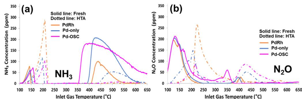
**Figure 3.** Effect of inlet gas temperature on the formation of (a) NH<sub>3</sub> and (b) N<sub>2</sub>O PdRh, Pd-only, and Pd-OSC fresh and HTA samples at stoichiometric condition.
