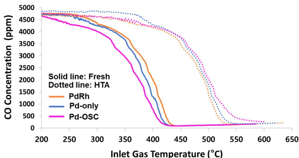
**Figure 4.** Conversion of CO in water–gas shift (WGS) reaction for PdRh, Pd-only, and Pd-OSC TWC fresh and HTA samples.
