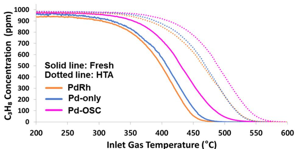
**Figure 5.** Conversion of  $C_3H_8$  in steam reforming (SR) reaction for PdRh, Pd-only, and Pd-OSC TWC fresh and HTA samples.
