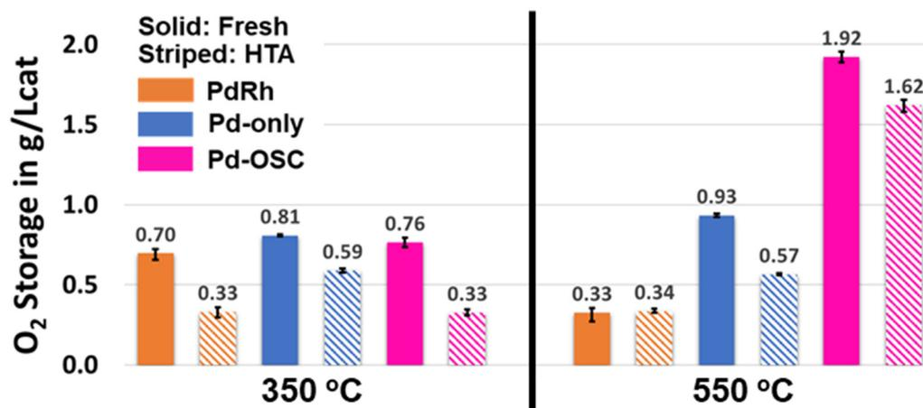
**Figure 1.** Oxygen storage capacity (OSC) for PdRh, Pd-only, and Pd-OSC TWC fresh (solid) and HTA (striped) samples.
