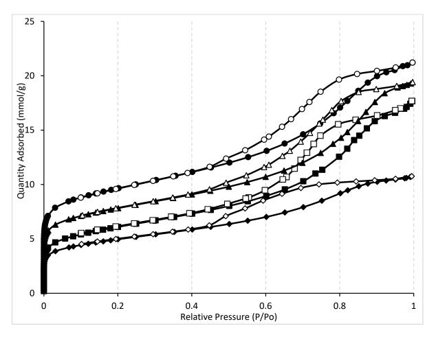
**Figure 2.** N<sub>2</sub>-adsorption–desorption isotherms measured at 77 K. for the catalysts Au@meso-UiO-66-before- ( $\bullet$ ) and -after-( $\blacktriangle$ ) catalysis nanohybrids; Au@meso-NH<sub>2</sub>-UiO-66-before- ( $\blacksquare$ ) and -after-catalysis nanohybrids ( $\blacklozenge$ ). (solid symbols—adsorption, open symbols—desorption).
