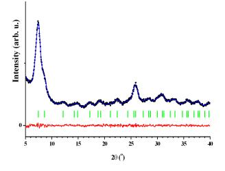
**Figure 6.** The Rietveld plot for the meso-UiO-66 material showing the experimental (black dots), calculated (blue) and difference (red) curves. The vertical green bars denote calculated positions of the peaks for the cubic crystal structure UiO-66.
