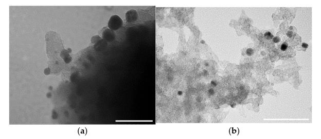
**Figure 4.** TEM micrographs of the (**a**) Au@meso-UiO-66-before-catalysis (scale bar is 100 nm) and (**b**) Au@meso-UiO-66-after-catalysis (scale bar is 50 nm) nanohybrids.
