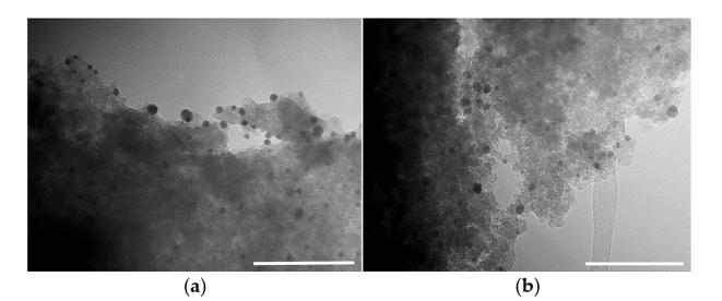
**Figure 5.** TEM micrographs of the (**a**) Au@meso-NH<sub>2</sub>-UiO-66-before-catalysis (scale bar is 100 nm) and (**b**) Au@meso-NH<sub>2</sub>-UiO-66-after-catalysis (scale bar is 200 nm) nanohybrids.
