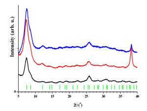
**Figure 8.** XRD patterns of the meso-UiO-66 (black), Au@meso-UiO-66-before-catalysis (red) and Au@meso-UiO-66-after-catalysis (blue) samples. The vertical bars denote calculated positions of the peaks for the cubic crystal structure UiO-66.
