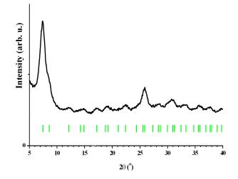
**Figure 7.** XRD powder pattern of the meso-NH<sub>2</sub>-UiO-66 sample. The vertical bars denote calculated positions of the peaks for the cubic crystal structure UiO-66.
