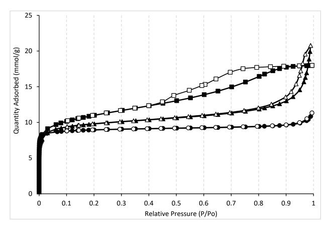
**Figure 1.** N<sub>2</sub>-adsorption–desorption isotherms measured at 77 K. for the micro-UiO-66 ( $\bullet$ ), meso-UiO-66 ( $\blacksquare$ ) and meso-NH<sub>2</sub>-UiO-66 ( $\blacktriangle$ ) materials (solid symbols—adsorption, open symbols—desorption) and Au@meso-NH<sub>2</sub>-UiO-66-before- and -after-catalysis nanohybrids.
