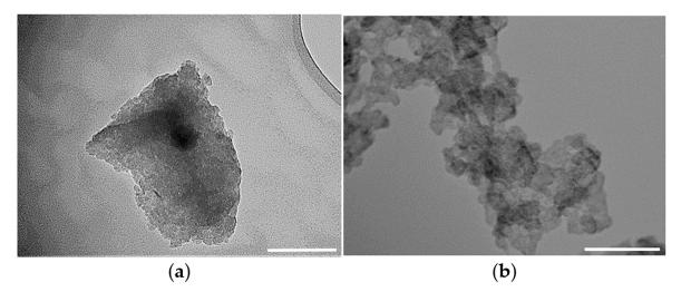
**Figure 3.** TEM micrographs of the pristine (**a**) meso-UiO-66 (scale bar is 200 nm) and (**b**) meso-NH<sub>2</sub>-UiO-66 (scale bar is 50 nm) materials.
