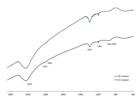
Figure 5. FTIR spectra of carbon materials after treatment with leaching solution (CCt and BCt).
