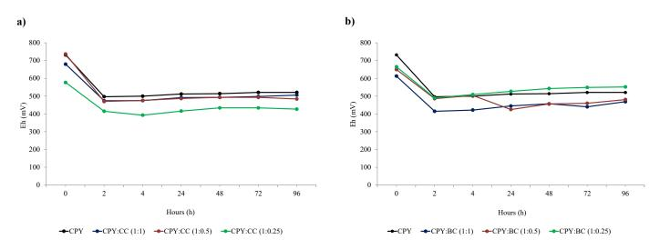
**Figure 6.** Eh (mV) evolution during leaching experiments with the addition of carbon materials: (a) CC and (b) BC.
