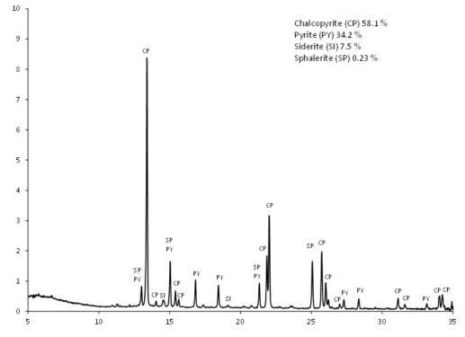
Figure 1. XRD pattern of CPY sample.
