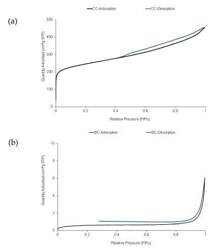
Figure 2.  $N_2$  isotherms of (a) CC and (b) BC carbon materials.
