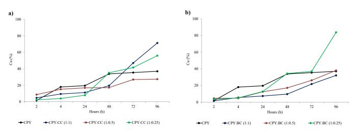
Figure 4. Evolution of copper extraction in the leaching solution: (a) CC and (b) BC.
