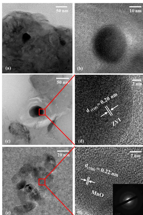
Figure 4. TEM images of (a,b) ZVI-C, (c) ZVI/Mn-C-31 and (e) Mn-C; HRTEM image of (d) ZVI/Mn-C-31 and (f) Mn-C. The inset in (f) shows the SAED pattern of Mn-C.
