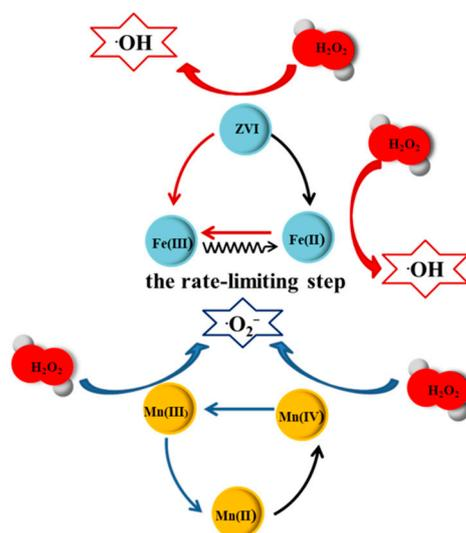
**Figure 12.** Proposed mechanism for the Fenton-like system over ZVI/Mn-C bimetallic catalyst.
