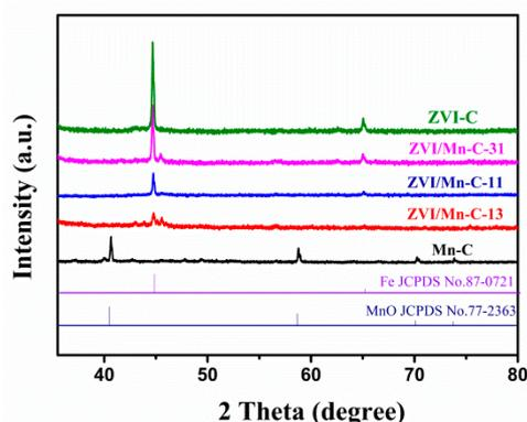
**Figure 2.** XRD patterns of ZVI/Mn-C samples.
