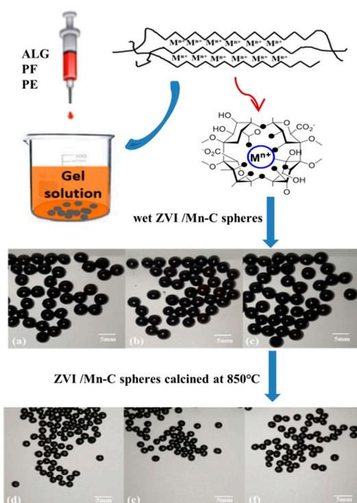
**Figure 1.** Schematic diagram of the preparation process for (a,d) ZVI/Mn-C-31, (b,e) ZVI/Mn-C-11, (c,f) ZVI/Mn-C-13.
