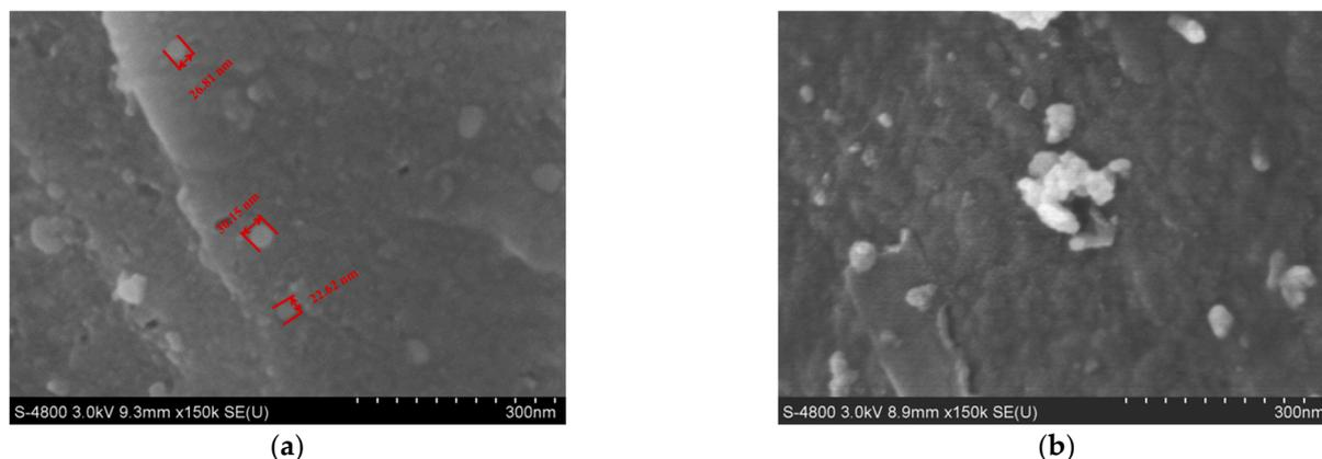
**Figure 10.** SEM images of ZVI/Mn-C-31 (a) before (b) after four reactions.
