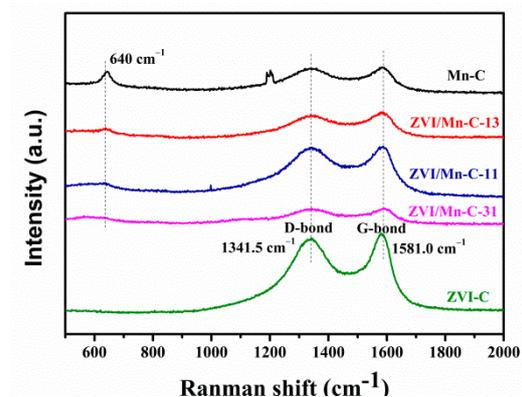
Figure 3. Raman spectra of ZVI/Mn-C samples.
