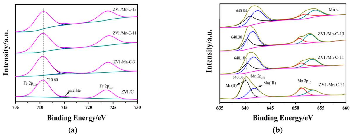
**Figure 5.** XPS spectra of (a) Fe 2p and (b) Mn 2p for all samples.
