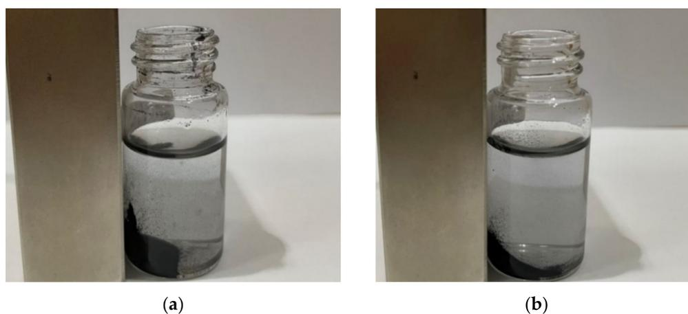
**Figure 8.** Magnetic separation of 0.5FePt/AC catalyst (a) after 1st cycle run and (b) after 3rd cycle run.
