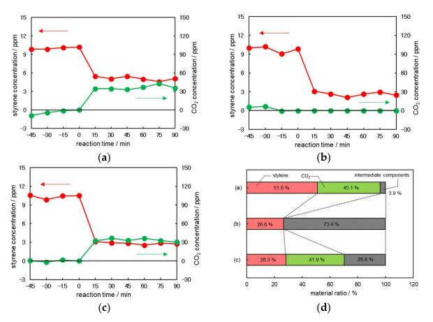
**Figure 4.** Typical data set of styrene removal (red) and  $CO_2$  generation (green) by reaction with (a) photocatalyst + UV irradiation, (b) ozone + UV irradiation, (c) photocatalyst + ozone + UV irradiation, and (d) carbon material balance for each reaction (red: unreacted styrene components, green: generated  $CO_2$  components, gray: generated intermediate components).
