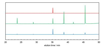
**Figure 5.** Gas chromatograms of gas components at reactor outlet by activated carbon tube solvent extraction method on each reaction (red: photocatalyst + UV irradiation, green: ozone + UV irradiation, blue: photocatalyst + ozone + UV irradiation).
