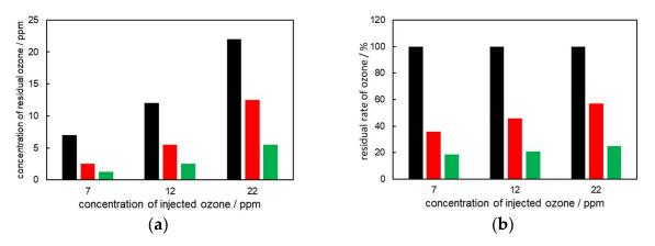
**Figure 6.** (a) Residual ozone concentration, (b) residual rate of ozone under each condition (black: without reaction, red: with ozone + UV irradiation, green: with photocatalyst + ozone + UV irradiation).
