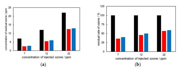
**Figure 3.** (a) Residual ozone concentration, (b) residual rate of ozone under each condition (black: without reaction, red: with UV irradiation, blue: without UV irradiation).
