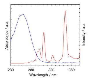
Figure 8. Spectrum of the spot light (red) and the ozone absorption curve (blue).
