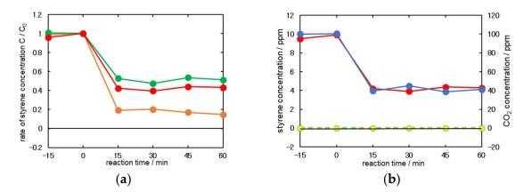
**Figure 1.** (a) Typical data set of styrene removal by reaction with each ozone concentration (green, red, and orange indicate 7 ppm, 12 ppm, and 22 ppm, respectively). (b) Typical data set of styrene removal (red, blue) and  $CO_2$  generation (green, yellow) by reaction with ozone (red, green: with UV irradiation, blue, yellow: without UV irradiation).
