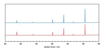
**Figure 2.** Gas chromatograms of gas components at reactor outlet by activated carbon tube–solvent extraction method (red: with ozone and UV irradiation, blue: with ozone only).
