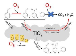
Figure 9. Proposed mechanisms of the decomposition of styrene using photocatalyst and ozone treatment.
