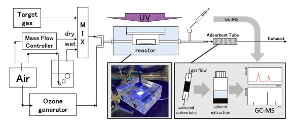
Figure 10. Photographs and schematic of evaluation equipment.
