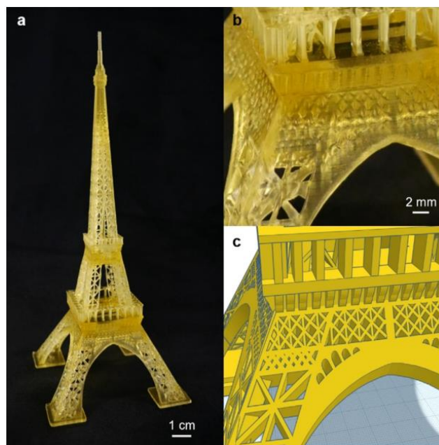
Figure 8. Eiffel Tower figurine that was 3D-printed using novel resins containing BTPA as RAFT agent. (a) Full-sized 3D-printed object; (b) close-up of 3D-printed figurine showing intricate, high-resolution details, and (c) the corresponding close-up of the original 3D model design. Object was printed using a ratio of [\text{BTPA}]:[\text{PEGDA}]:[\text{DMAM}]:[\text{TPO}] = 1:40:160:2 under violet light ( \lambda_{\text{max}} = 405 \text{ nm} , I_0 = 0.81 \text{ mW cm}^{-2} ) irradiation. Adapted from [69] with permission from Wiley.
