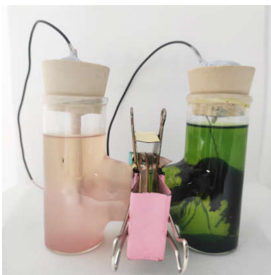
Figure S10. Dual-chamber MFC device
