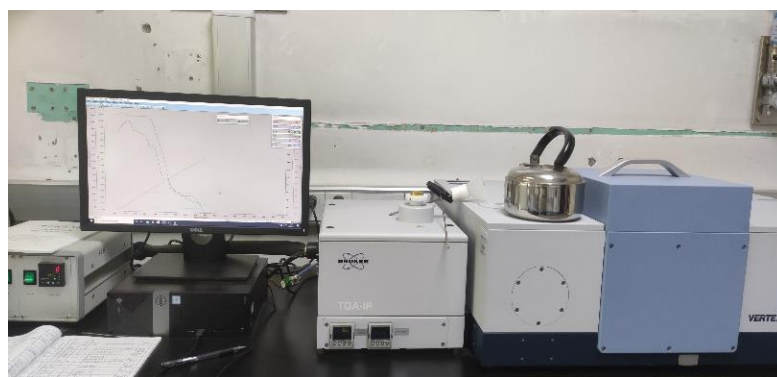
Figure S9 The thermogravimetric analyzer (Sta 449F3, Netzsch, Germany) coupled to an FTIR spectrometer (Vertex80v, Bruker, Germany)
