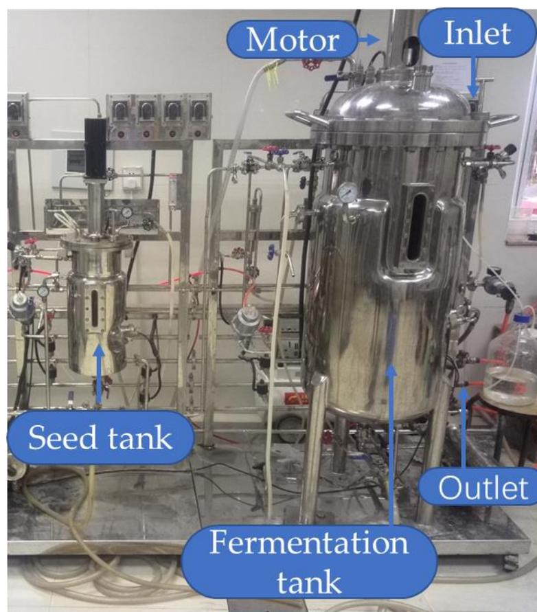
**Figure 8.** Pilot-scale experimental set-up (100 L).
