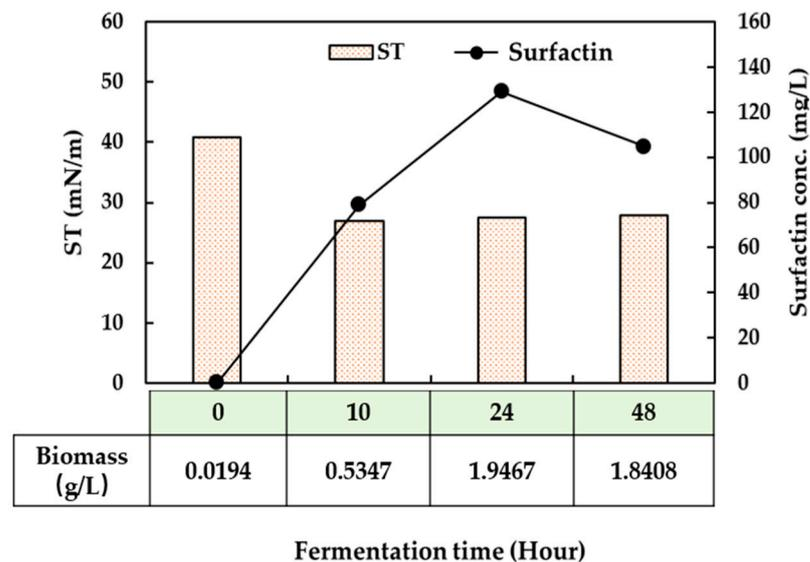
**Figure 4.** ST values, surfactin concentrations, and biomass in pilot-scale experiments (100 L).
