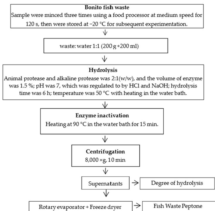
**Figure 6.** Flow chart of the enzyme hydrolysis in the laboratory.
