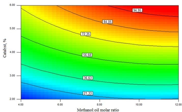
**Figure 6.** Response surface contour plot for the interaction between the catalyst amount and the methanol-to-oil ratio for the ester yield when the process temperature is 64 °C and the process duration is 5 h.
