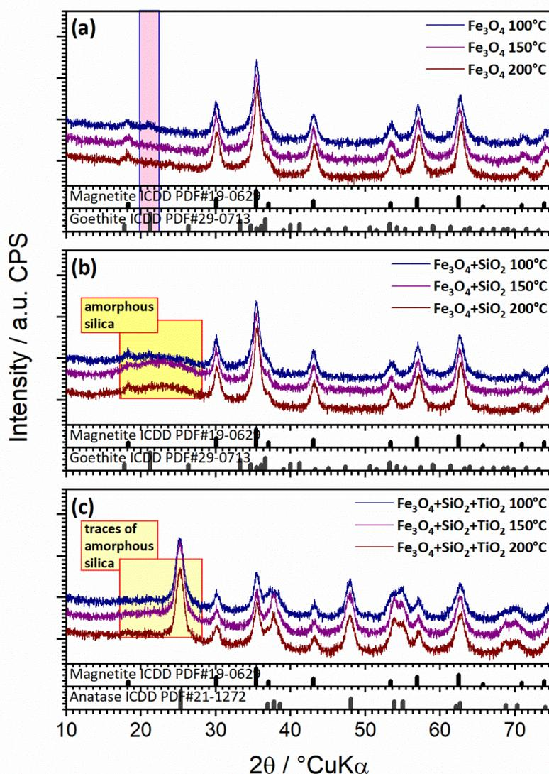
**Figure 2.** Diffractograms of  $\text{Fe}_3\text{O}_4$  (a),  $\text{Fe}_3\text{O}_4/\text{SiO}_2$  (b), and  $\text{Fe}_3\text{O}_4/\text{SiO}_2/\text{TiO}_2$  (c) samples synthesized by the microwave-assisted method at 100 °C (blue line), 150 °C (violet line), and 200 °C (brown line).
