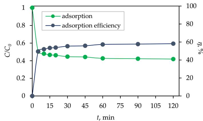
**Figure 5.** Dark adsorption and adsorption efficiency ( $\eta$ ; %) of ciprofloxacin (CIP) by  $\text{Fe}_3\text{O}_4/\text{SiO}_2/\text{TiO}_2$  nanocomposites synthesized at  $100^\circ\text{C}$  as a function of time ( $c$  (CIP) =  $10 \text{ mg dm}^{-3}$ ,  $V$  (CIP) =  $100 \text{ cm}^3$ ,  $m$  (core-shell photocatalyst) =  $50 \text{ mg}$ , and  $T = 25^\circ\text{C}$ ).
