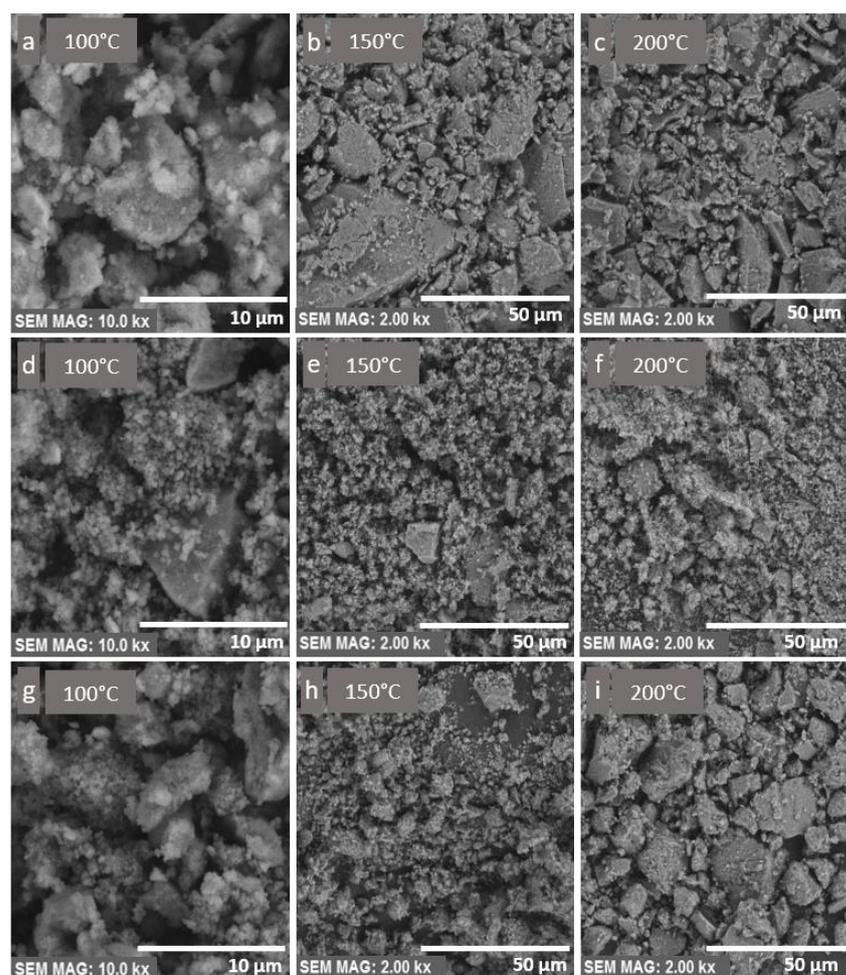
**Figure 4.** (a–c) SEM images of  $\text{Fe}_3\text{O}_4$  nanocomposites synthesized by the microwave-assisted method at 100, 150, and 200 °C, respectively. (d–f) SEM images of  $\text{Fe}_3\text{O}_4/\text{SiO}_2$  nanocomposites synthesized by the microwave-assisted method at 100, 150, and 200 °C, respectively. (g–i) SEM images of  $\text{Fe}_3\text{O}_4/\text{SiO}_2/\text{TiO}_2$  nanocomposites synthesized by the microwave-assisted method at 100, 150, and 200 °C, respectively.
