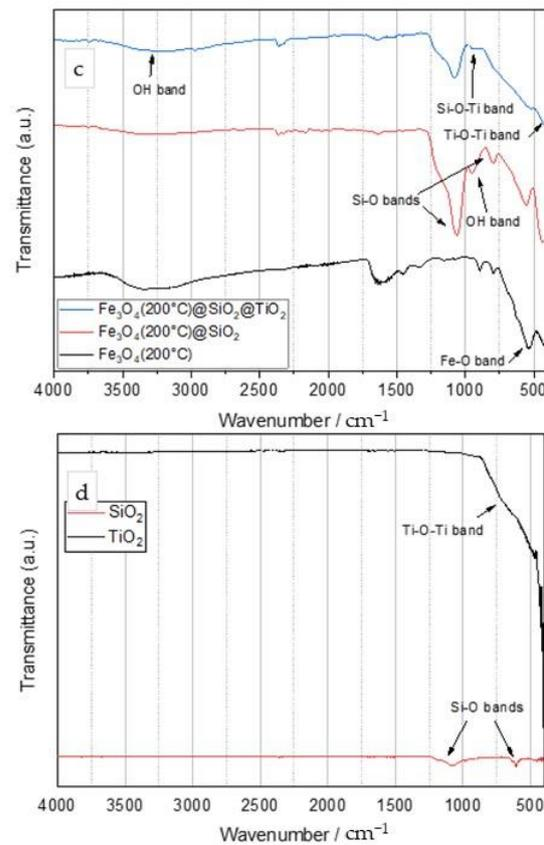
**Figure 1.** FTIR spectra of  $\text{Fe}_3\text{O}_4$  (black line),  $\text{Fe}_3\text{O}_4/\text{SiO}_2$  (red line), and  $\text{Fe}_3\text{O}_4/\text{SiO}_2/\text{TiO}_2$  (blue line) particles synthesized by the microwave-assisted method at 100 °C (a), 150 °C (b), and 200 °C (c). (d) FTIR spectra of pure  $\text{TiO}_2$  and  $\text{SiO}_2$ .
