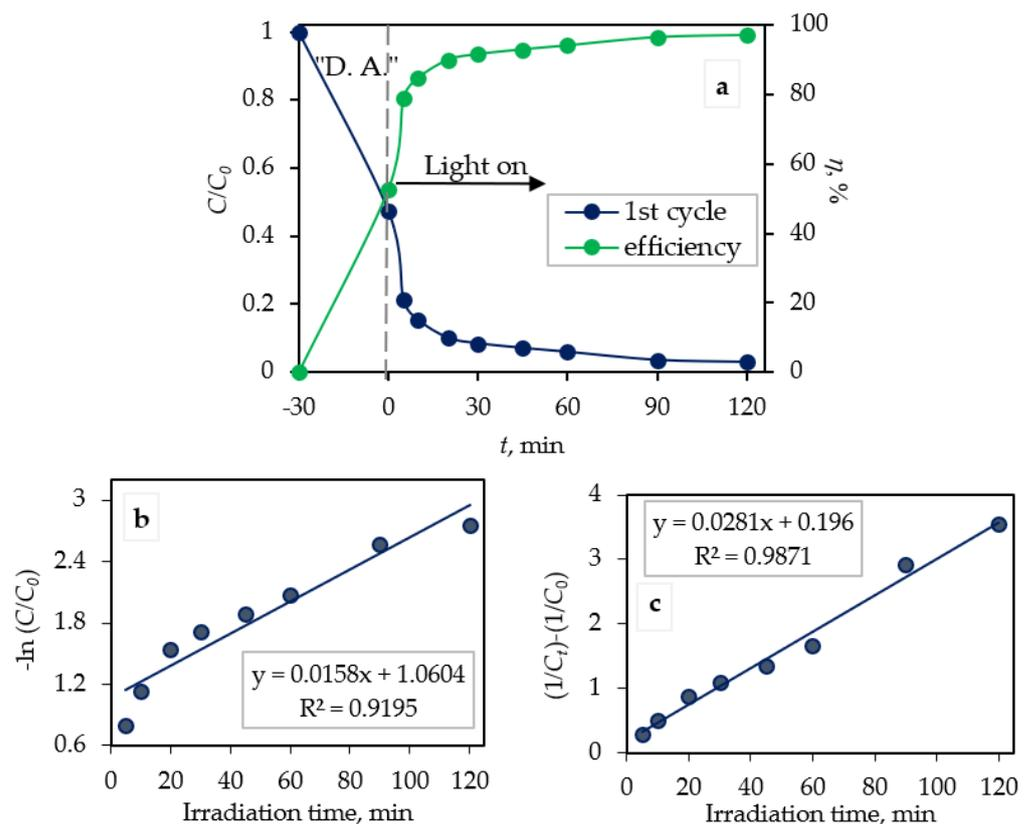
**Figure 9.** (a) Photocatalytic degradation of CIP by the  $\text{Fe}_3\text{O}_4/\text{SiO}_2/\text{TiO}_2$  nanocomposite synthesized at  $100^\circ\text{C}$  monitored via UV/VIS spectrophotometry. The pseudo-first-order plot (b) and the pseudo-second-order plot (c) of CIP photocatalytic degradation.
