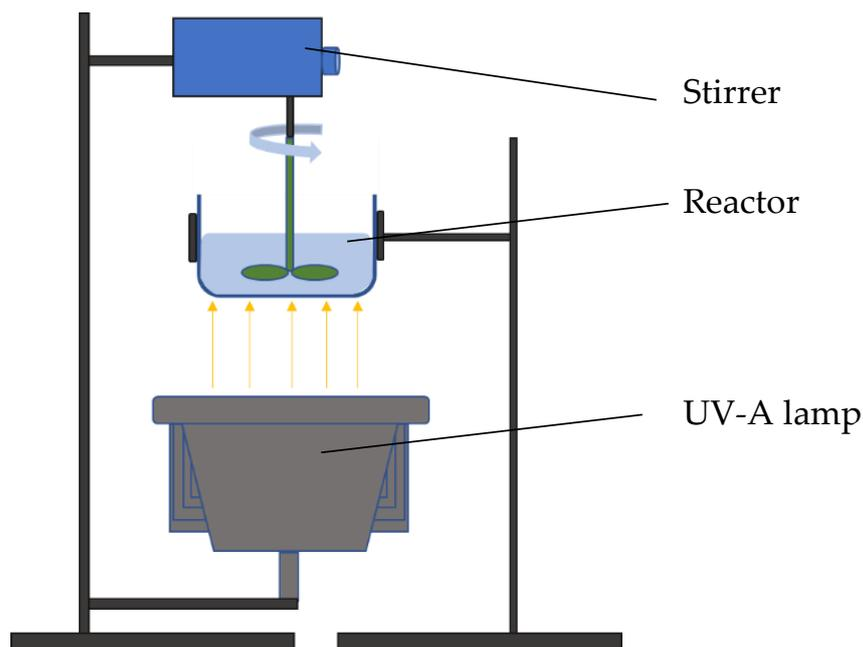
**Figure 11.** The reactor for photocatalytic measurements.
