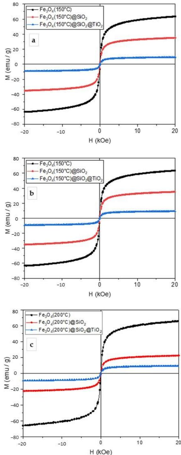
**Figure 3.** Magnetization curves of  $\text{Fe}_3\text{O}_4$ ,  $\text{Fe}_3\text{O}_4/\text{SiO}_2$ , and  $\text{Fe}_3\text{O}_4/\text{SiO}_2/\text{TiO}_2$  nanoparticles synthesized by the microwave-assisted method at 100 °C (a), 150 °C (b), and 200 °C (c).
