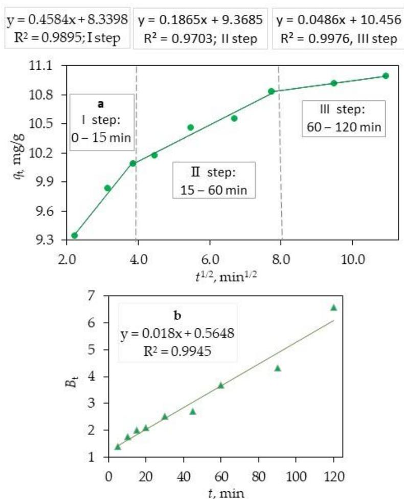
**Figure 7.** The adsorption kinetic data of CIP on the ternary core-shell  $\text{Fe}_3\text{O}_4/\text{SiO}_2/\text{TiO}_2$  nanocomposite fitted with Webe–Morris intraparticle diffusion (a) and Boyd diffusion models (b).
