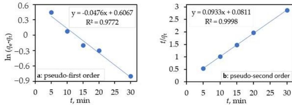
**Figure 6.** Pseudo-first-order plots (a) and pseudo-second order plot (b) of the adsorption of CIP on the ternary core–shell  $\text{Fe}_3\text{O}_4/\text{SiO}_2/\text{TiO}_2$  nanocomposite ( $c$  (CIP) =  $10 \text{ mg dm}^{-3}$ ,  $V$  (CIP) =  $100 \text{ cm}^3$ ,  $m$  (core–shell photocatalyst) =  $50 \text{ mg}$ , and  $T = 25 \text{ }^\circ\text{C}$ ).
