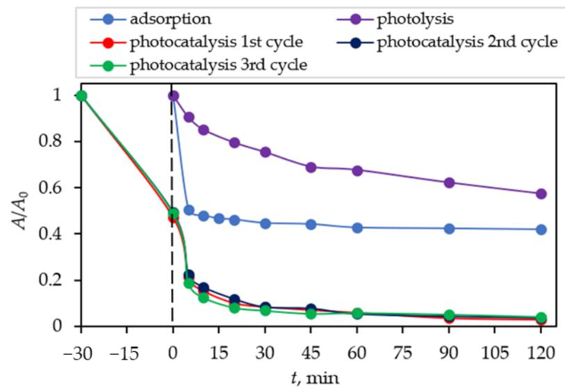
**Figure 8.** Dark adsorption and photolytic and photocatalytic degradation of CIP as a function of irradiation time by the  $\text{Fe}_3\text{O}_4/\text{SiO}_2/\text{TiO}_2$  nanocomposite synthesized at  $100^\circ\text{C}$ .
