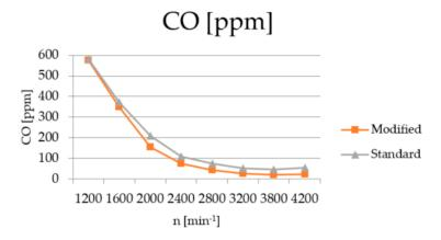
**Figure 14.** Carbon monoxide CO measurement results for the standard CR system and the modified CR system. Measurement error of exhaust fumes analyzer 1.5%.
