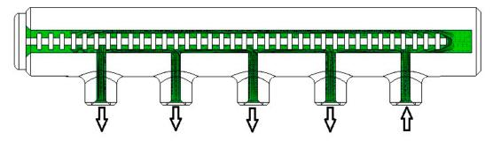
Figure 5. Simulation of fuel flow through CR.
