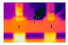
Figure 11. Temperature distribution tests in atomizers: (1) modified; (2) standard.
