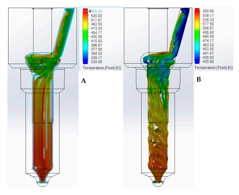
Figure 7. The results of preliminary simulation studies of the flow and temperature distribution of the fuel through the standard and modified atomizer. Flow parameters: injection dose:  $35.3 \text{ mm}^3/\text{H}$ , injection time:  $780 \mu \text{s}$ , pressure in the system: 135 MPa. (A) Standard atomizer; (B) modified atomizer.
