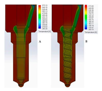
**Figure 10.** The results of preliminary simulation studies of temperature distribution of body and needle at the pressure of 135 MPa. (A) Standard atomizer; (B) modified atomizer.
