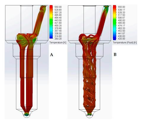
**Figure 9.** The results of preliminary simulation studies of the flow and temperature distribution of the fuel through the standard and modified atomizer. Flow parameters: injection dose:  $1.2 \text{ mm}^3/\text{H}$ , injection time:  $260 \mu \text{s}$ , pressure in the system: 80 MPa. (A) Standard atomizer; (B) modified atomizer.
