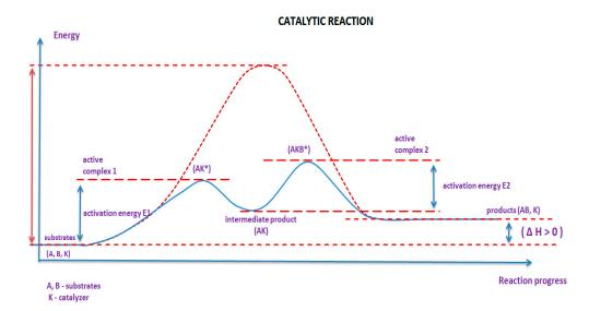
**Figure 3.** Course of chemical reaction with catalyst.
