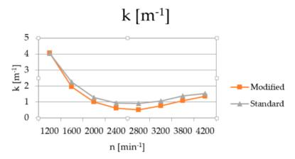
**Figure 15.** Exhaust fumes results for the standard CR system and the modified CR system Measurement error of the opacimeter: 2%.
