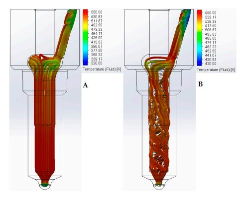
**Figure 8.** The results of preliminary simulation studies of the flow and temperature distribution of the fuel through the standard and modified atomizer. Flow parameters: injection dose:  $0.7 \text{ mm}^3/\text{H}$ , injection time:  $420 \, \mu\text{s}$ , pressure in the system:  $30 \, \text{MPa}$ . (A) Standard atomizer; (B) modified atomizer.
