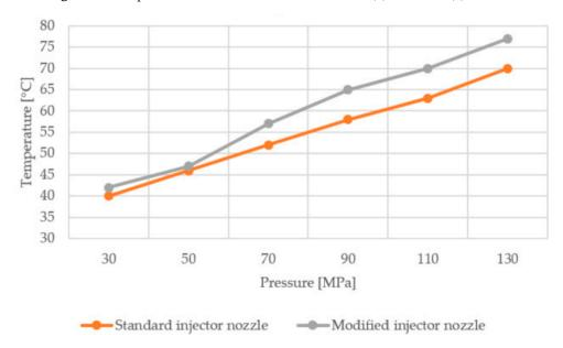
**Figure 12.** Fuel temperature results at the discharge from the atomizer with different pressures in the system.
