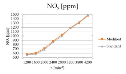
Figure 13. Results of nitrogen oxide  $NO_X$  measurements for the standard CR system and the modified CR system.
