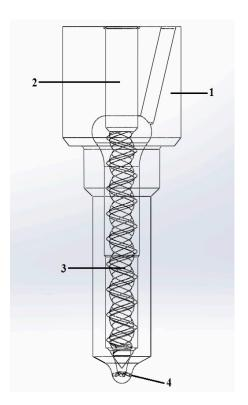
**Figure 2.** Modified fuel injector atomizer: 1—case, 2—precise needle pair, 3—spiral-elliptical channels made on the inoperative part of the needle with a catalytic reactor, 4—injection holes.
