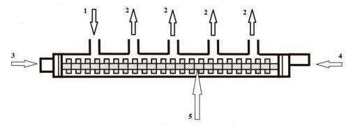
**Figure 1.** Modified common rail (CR) high-pressure battery: 1—fuel supply to the rail, 2—output for fuel injectors, 3—high-pressure sensor, 4—high-pressure regulator, 5—catalytic reactor.
