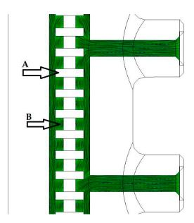
Figure 6. Common rail with catalyst. (A) Catalyst reactor; (B) fuel flowing through the reactor.
