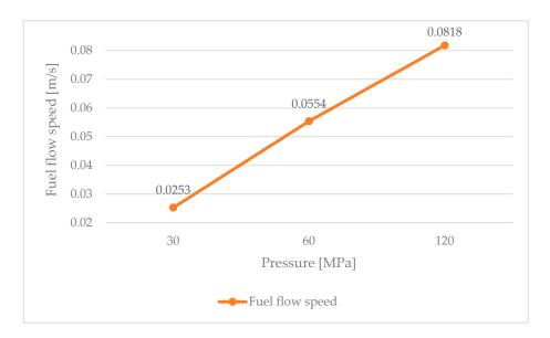
Figure 4. Fuel flow speed inside the injector nozzle depends on the system pressure [19].
