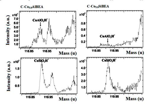
Figure 4. ToF-SIMS spectra of  $CoAlO_2H^+$  and  $CoSiO_2H^+$  ions collected for C-Co<sub>5.0</sub>AlBEA and C-Co<sub>5.0</sub>SiBEA.
