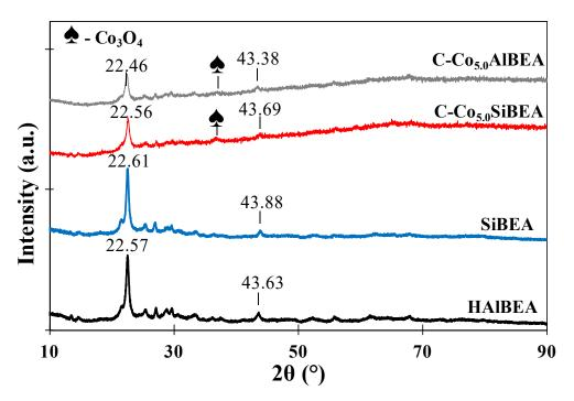
**Figure 1.** XRD diffractograms of HAlBEA, SiBEA, C-Co<sub>5.0</sub>AlBEA and C-Co<sub>5.0</sub>SiBEA showing contraction of the zeolite matrix after dealumination and expansion after incorporation of Co cations.
