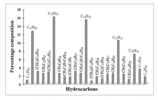
**Figure 11.** GC- MS analysis of liquid products obtained in FTS on Red-C-Co<sub>5.0</sub>SiBEA catalyst reduced at 900  $^{\circ}$ C in 5% H<sub>2</sub>-95% Ar flow.
