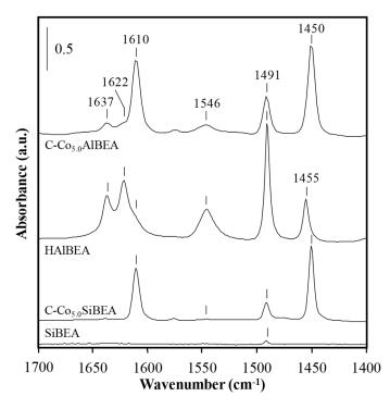
**Figure 7.** FTIR spectra of AlBEA, SiBEA, Co<sub>5.0</sub>AlBEA and Co<sub>5.0</sub>SiBEA after desorption of pyridine at 150 °C showing no Brønsted and Lewis acidic sites in siliceous SiBEA.
