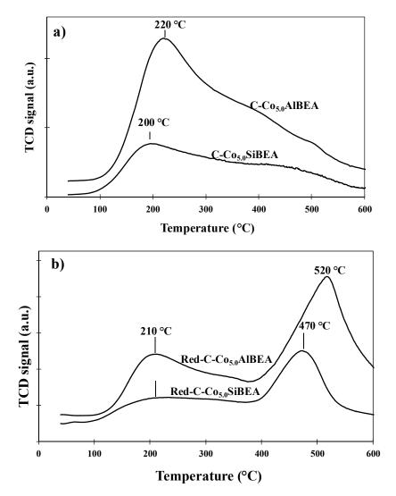
**Figure 6.** TPD-NH<sub>3</sub> patterns for C-Co<sub>5.0</sub>AlBEA and C-Co<sub>5.0</sub>SiBEA (**a**) and Red-C-Co<sub>5.0</sub>AlBEA and Red-C-Co<sub>5.0</sub>SiBEA reduced in H<sub>2</sub> at 500 °C for 1 h (**b**).
