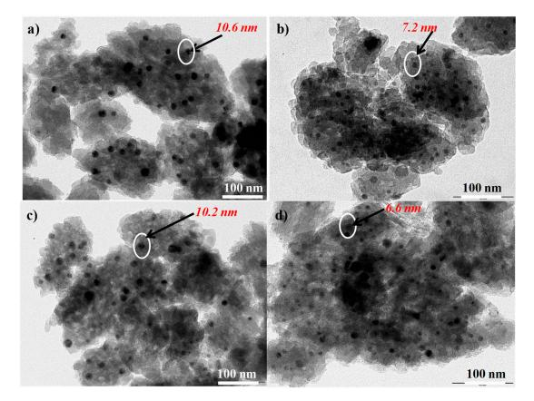
**Figure 5.** TEM EDS images of Red-C-Co<sub>5.0</sub>SiBEA reduced at 800 °C in 5% H<sub>2</sub>-95% Ar flow (**a**), 100% H<sub>2</sub> flow (**b**), 900 °C in 5% H<sub>2</sub>-95% Ar flow (**c**), 100% H<sub>2</sub> flow (**d**) showing that the size of cobalt nanoparticles does not change after reduction in higher temperature.
