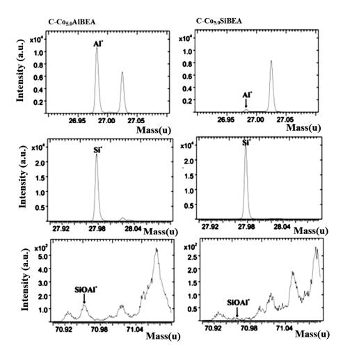
Figure 3. ToF-SIMS spectra of Al<sup>+</sup>, Si<sup>+</sup> and SiOAl<sup>+</sup> ions collected for C-Co<sub>5.0</sub>AlBEA and C-Co<sub>5.0</sub>SiBEA.
