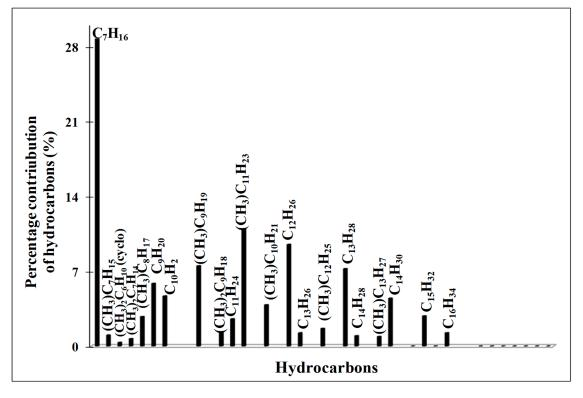
**Figure 8.** GC–MS analysis of liquid products obtained in FTS on Red-C-Co<sub>5.0</sub>SiBEA catalyst reduced at 500  $^{\circ}$ C in 100% H<sub>2</sub> flow.
