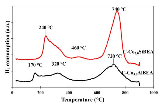
**Figure 2.** TPR-H<sub>2</sub> profiles of C-Co<sub>5.0</sub>AlBEA and C-Co<sub>5.0</sub>SiBEA performed in the temperature between 25 and 900 °C showing that C-Co<sub>5.0</sub>SiBEA is hardly reduced than C-Co<sub>5.0</sub>AlBEA.
