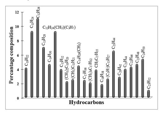
**Figure 9.** GC–MS analysis of liquid products obtained in FTS on Red-C-Co<sub>5.0</sub>SiBEA catalyst reduced at 800  $^{\circ}$ C in 100% H<sub>2</sub> flow.
