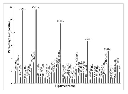
**Figure 10.** GC-MS analysis of liquid products obtained in FTS on Red-C-Co<sub>5.0</sub>SiBEA catalyst reduced at 900 °C in 100%  $H_2$  flow.
